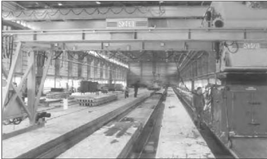
Figure 2.7: Long line prestressed extrusion of hollow core floor slabs (courtesy Spaecom Betonfertigteile GmbH & Co. KG., Germany).
