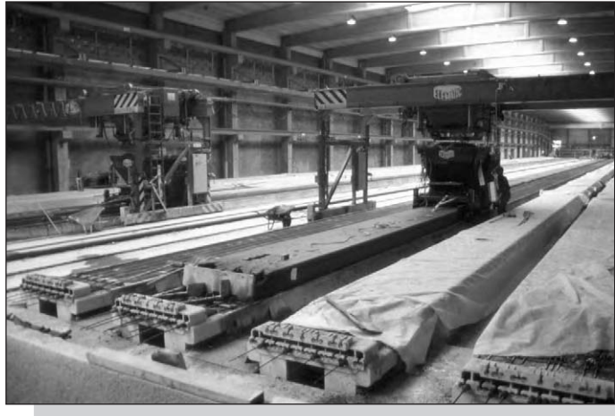
Figure 4.16: Production factory for hollow core floor units.
