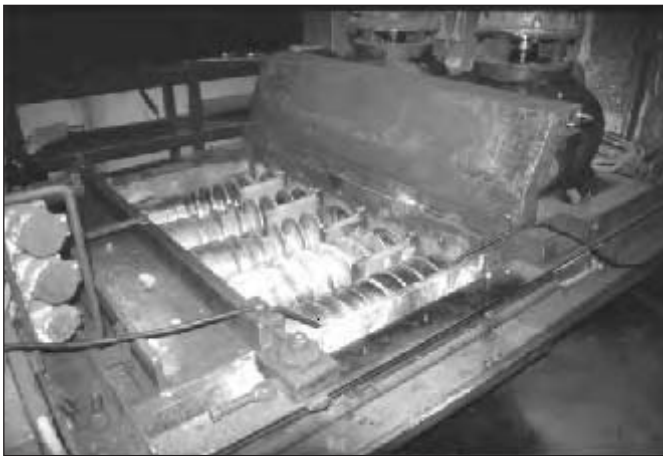
Figure 2.5: Rotating augers create forced extrusion of concrete.
