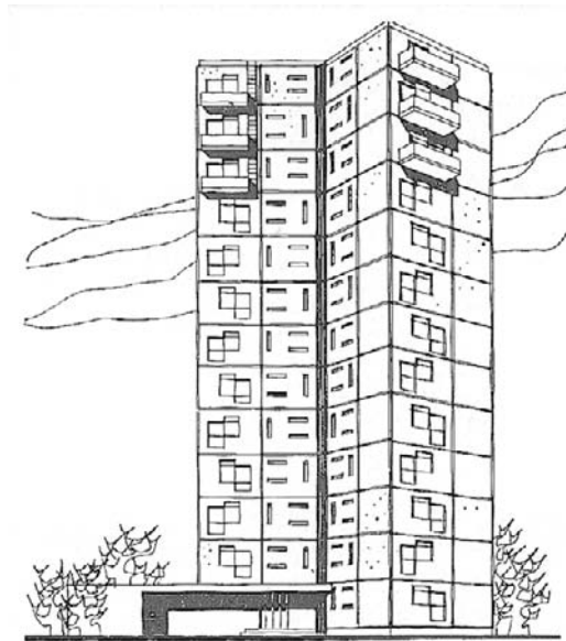
Figure 1.7 Large Panel Building, System Camus, Pantin near Paris, France. System building with room-sized large panels became a new form of industrialization in certain countries and for some time. © Sebestyen: Large Panel Buildings , Akadémiai Kiadó.
