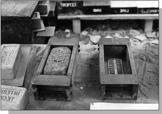
Figure 8.8: Wooden mould for handmade bricks.
