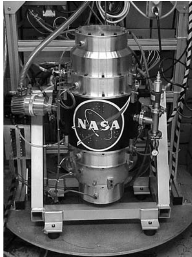
A NASA-developed flywheel energy storage
