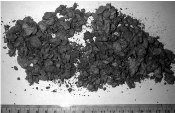
A potentially useful by-product is anaerobic digestate (Reproduced with permission from Alex Marshall, Clarke Energy Ltd)
