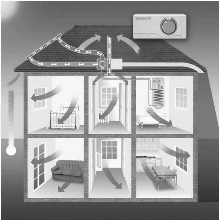
The Sunwarm system uses solar heated air for space heating and DHW (Reproduced with permission from Nuairé)
