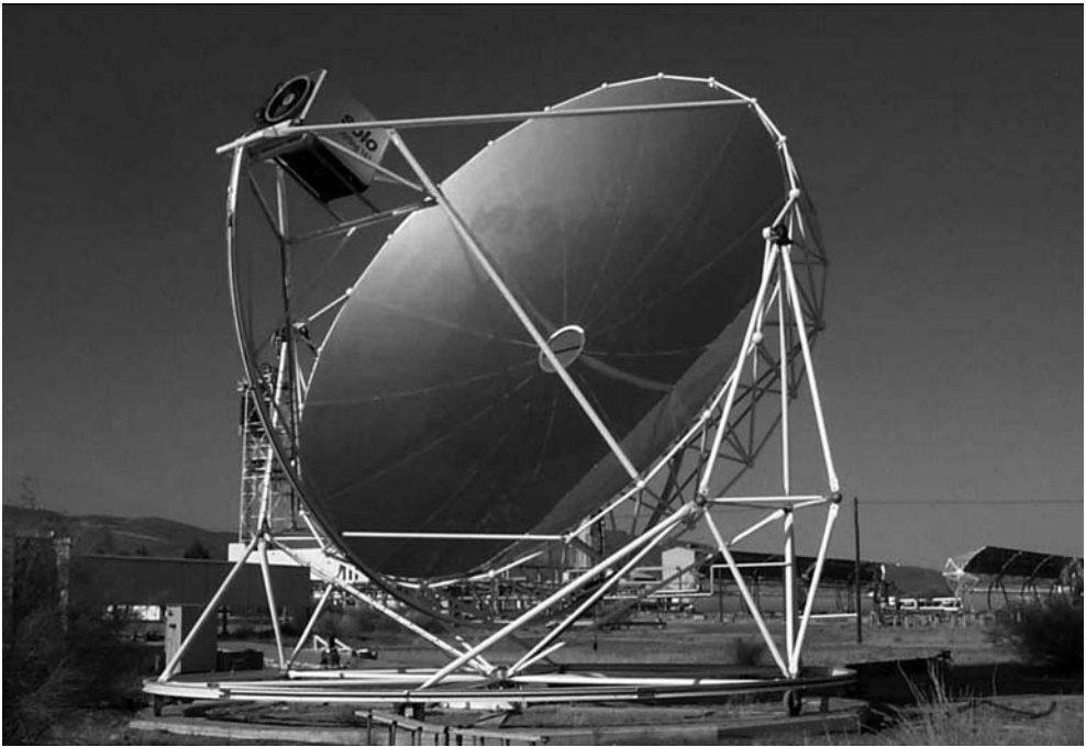
Using a concentration mirror to focus sunlight onto a Stirling engine is still at the experimental stage (credit Schlaich Bergermann and Partner)
