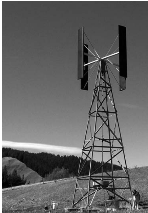
VAWTs can be mounted on towers, as shown by this 4 blade, 6 kW Solwind unit (Reproduced with permission from Alvesta)
