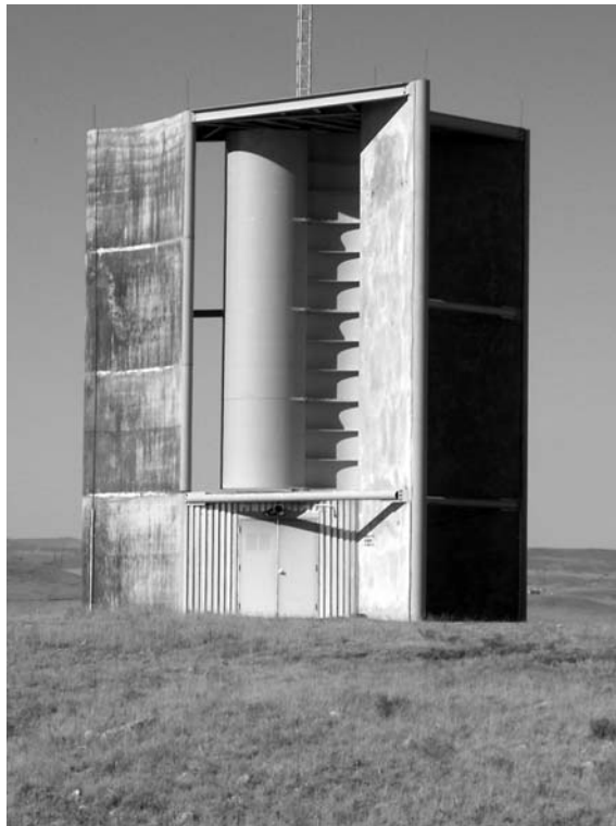
An original approach to VAWT design – the 2007 version of the TMA unit (Reproduced with permission from TMA Wind)
