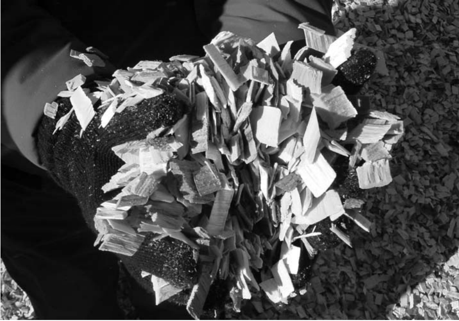
Moisture content of woodchips is critical (Reproduced with permission from Biomass Energy Centre)
