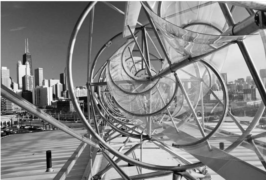
Aerotecture's 520H Aeroturbine is one recent example of a VAWT turned on its side to better integrate with the building (Reproduced with permission from Kurt Holtz, Lucid Dreams Productions)
