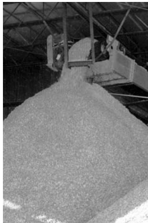
Large volumes of damp woodchip can pose the risk of spontaneous combustion (Reproduced with permission from Biomass Energy Centre)
