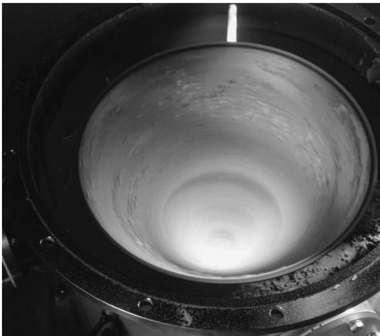
A rotating cone pyrolysis reactor (Reproduced with permission from Biomass Technology Group)
