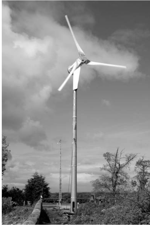
An established downwind HAWT – the 15kW Proven 15 (Reproduced with permission from Proven Energy)
