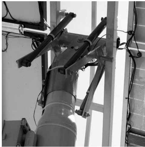
A passive solar tracking mechanism (Reproduced with permission from Leonard G.)
