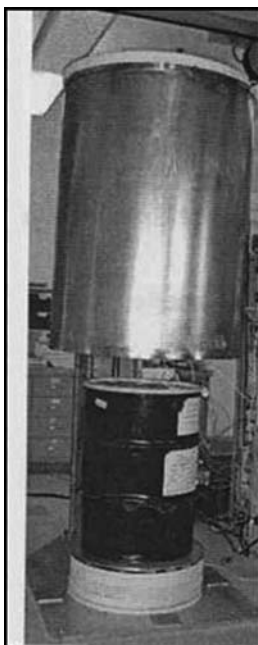
FIGURE 3A.27 Photograph of the LVC with the calorimeter in the up position to enable loading the 208-L drum.
