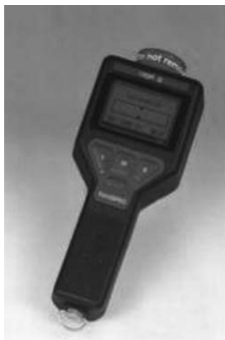
FIGURE 3A.29 The FieldSPEC is a handheld NaI \gamma -ray spectrometer with digital signal processing, gain stabilization, 8+ hour battery life, and full multichannel analyzer (MCA) capability.
