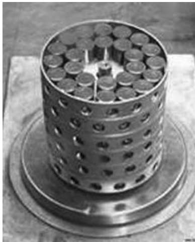
FIGURE 19.4 MOX fuel pellets. (Photo credit: Los Alamos National Laboratory and National Nuclear Security Administration.)
