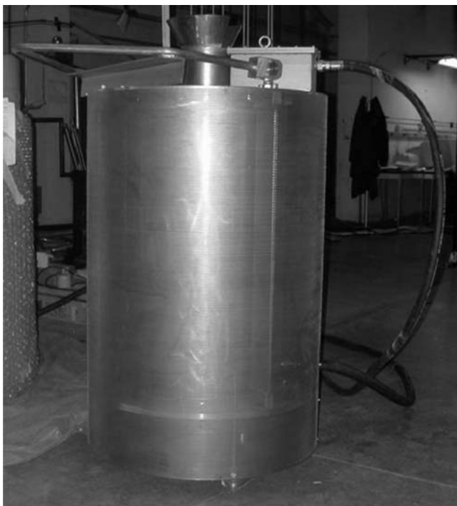
FIGURE 3B.4 The Research Reactor Fuel Counter (RRFC-II) shown at poolside.
