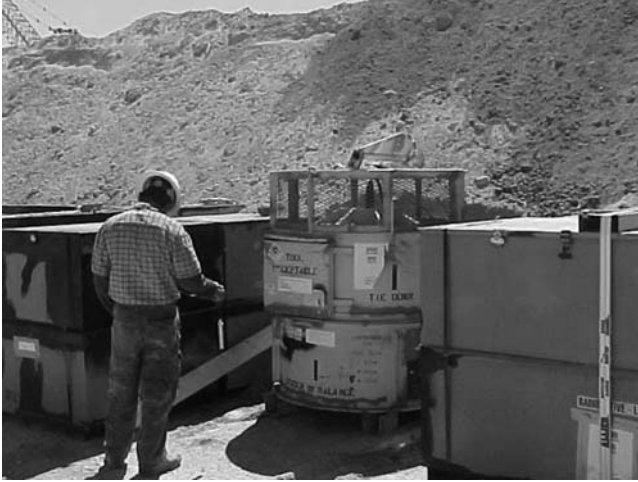
FIGURE 25.7 The rounded unit in the center of the photo is an RTG containing approximately 15,000 curies of strontium-90 after 30 years of decay. This unit is being buried at the DOE low-level waste disposal facility at the Nevada Test Site. (Photo supplied by Los Alamos National Laboratory Off-Site Source Recovery Project.)
