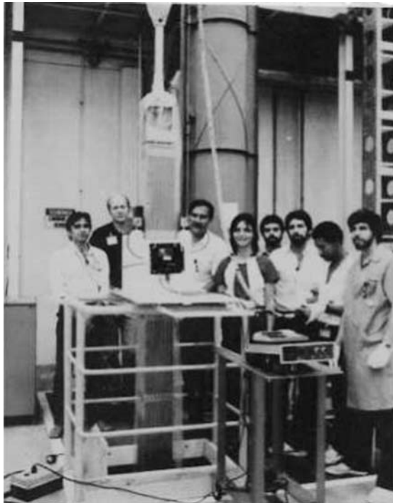
FIGURE 3A.20 The uranium neutron coincidence collar in use at Resende, Brazil, to measure PWR fuel assemblies.
