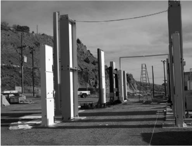
FIGURE 26.6 Radiation portal monitors being readied for simultaneous testing. Six vendors are represented.
