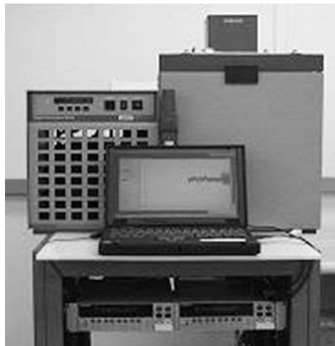
FIGURE 3A.26 Picture of a high-precision, solid-state calorimeter in a water bath. The laptop is used for data acquisition.
