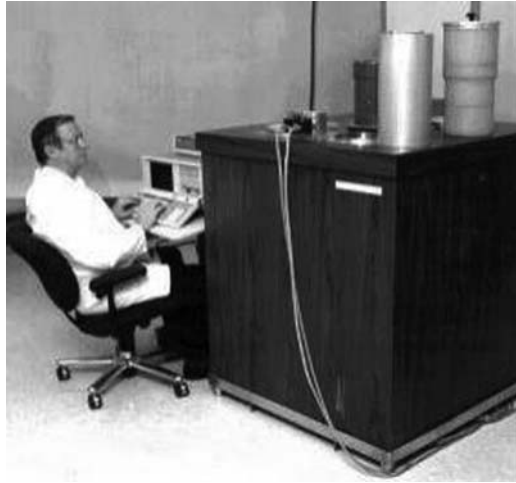
FIGURE 3A.25 A twin-bridge, heat-flow calorimeter. The large block is the water bath. The calorimeter can and the insulating plug rest on top of the water bath.
