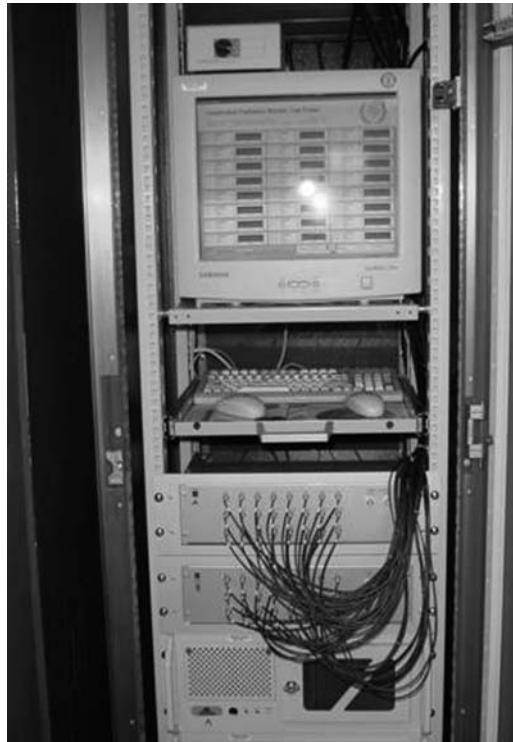
FIGURE 6.14 UMS signal generator for testing radiation-based systems.
