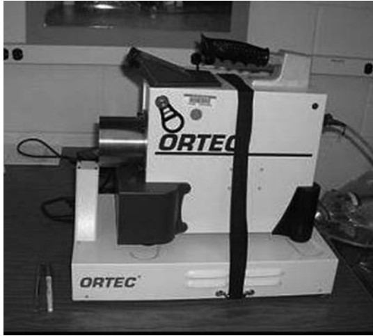
FIGURE 3A.31 The ORTEC Detective is shown mounted on a docking station used for charging, calibration, and cool-down. A small ^{137}\text{Cs} source is mounted inside the docking station.
