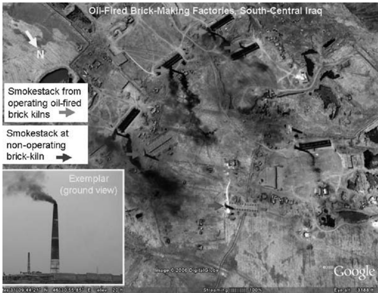
FIGURE 12.2 Numerous, innocuous (and air-polluting) oil-fired brickmaking kilns are present on this image that are a common feature in the developing world, but not necessarily a familiar one to most nonproliferation imagery analysts. Also be aware that, although nuclear facilities frequently contain ventilation stacks that are never intended to exhaust “smoke,” a smokestack may be present at, or near, a nuclear facility in association with a supporting thermal (conventional) power plant or steam plant.
