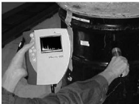
FIGURE 3A.30 The Canberra InSpector 1000 measuring a 208-L drum. The NaI detector fits in the right side of the electronics package.
