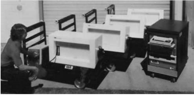
FIGURE 3C.8 Wide-area neutron detectors used to measure holdup at gaseous diffusion enrichment plants.
