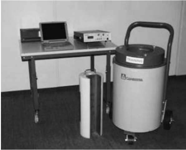
FIGURE 3A.19 An active well coincidence counter (AWCC) that uses two AmLi sources to induce fission in ^{235}\text{U} . It can assay kg quantities of HEU to a precision of 1–5% in 1,000s. It can also measure LEU oxide or pellets to 5–10% in 1,000s. The polyethylene cylinder on the left is an insert for measuring MTR fuel assemblies.
