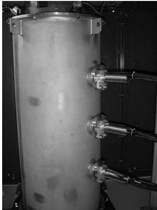
FIGURE 9.3 iPCAS with germanium detectors and neutron coincidence counter.
