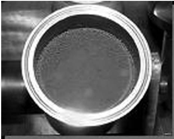
FIGURE 19.3 Canister of mixed oxide. (Photo credit: Los Alamos National Laboratory and National Nuclear Security Administration.)
