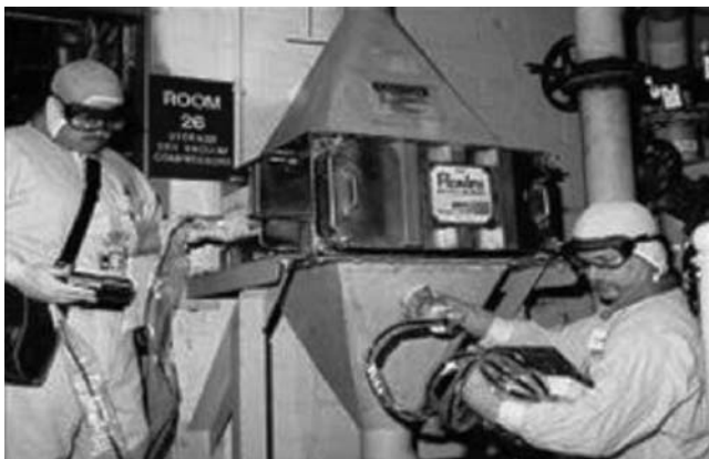
FIGURE 3C.5 Measurements of ^{235}\text{U} deposits in a filter system performed with CZT and NaI.
