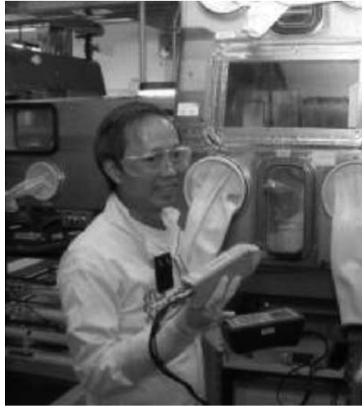
FIGURE 3C.1 The Peltier-cooled CdTe detector is shown measuring Pu isotopics in a glove box.
