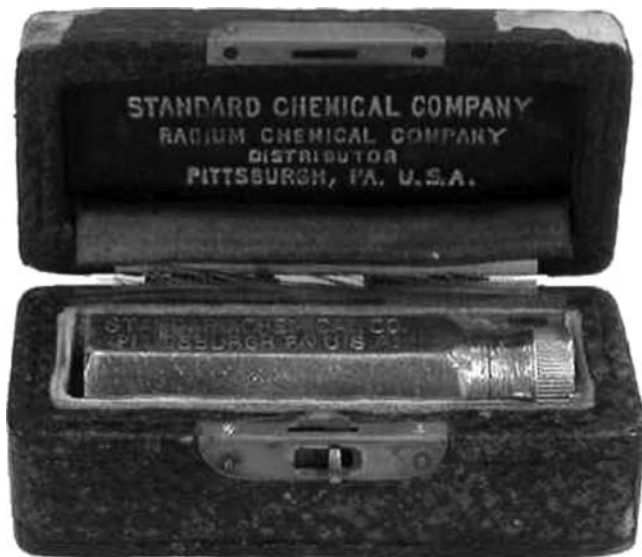
FIGURE 25.1 Radium-226 cancer therapy kit containing a lead shield to hold radium needles, circa 1920 to 1940. (Photo from Oak Ridge Associated Universities Website Museum.)
