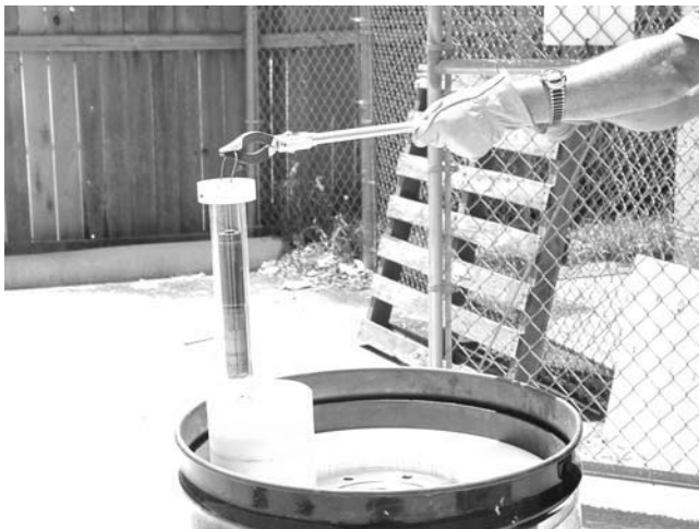
FIGURE 25.5 Two excess 16-curie americium-241 well-logging neutron generators are placed in a shielded container for recovery and removal to Los Alamos National Laboratory under NNSA/GTRI Programs. (Photo supplied by Los Alamos National Laboratory Off-Site Source Recovery Project.)
