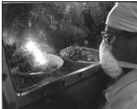
FIGURE 19.1 HEU monitor at Russian facility used to burn uranium metal and produce uranium oxide. (Photo credit: Lawrence Livermore National Laboratory.)
