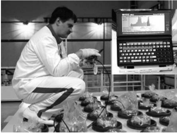
FIGURE 5.4 Using CdZnTe detector to measure uranium spectrum in fresh LEU fuel.
