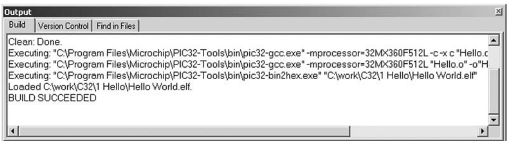
Figure 1.2: The content of the Output Window Build tab after a successful build.
