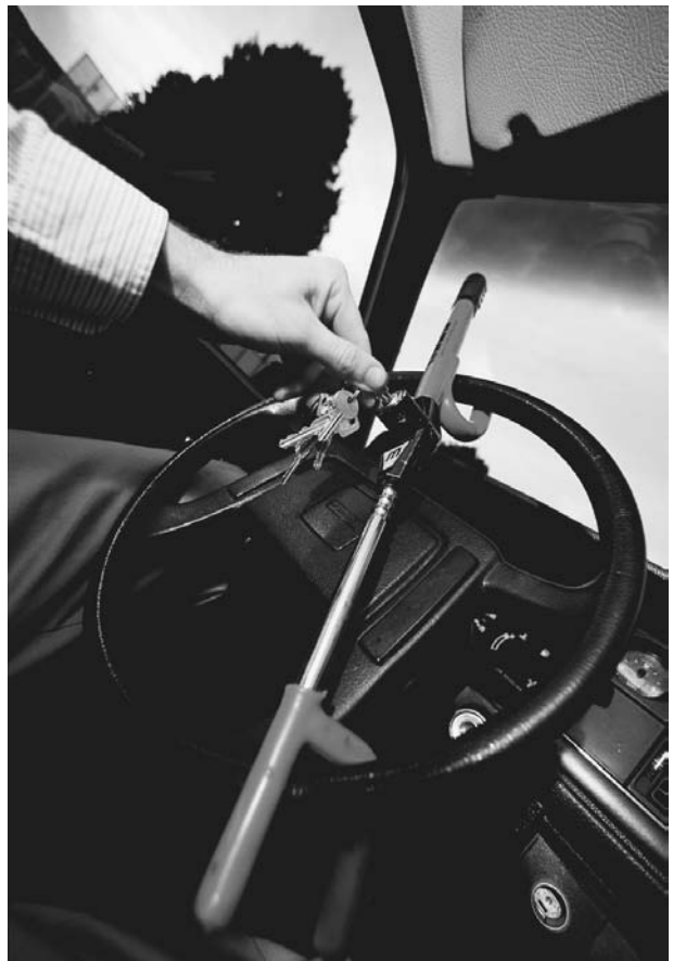
A device called “The Club” locks the steering wheel in place and is a good deterrent to theft. (© David Butow/Corbis)
