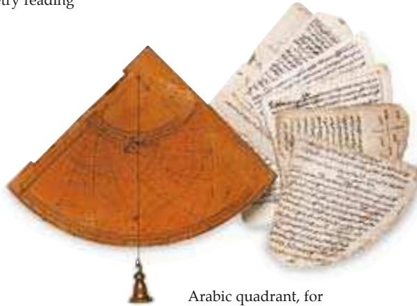
Arabic quadrant, for measuring the height of stars, with instructions
