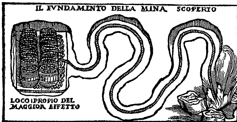
Fig. 9. Gunpowder mine with zigzag passage containing the fuse (Biringuccio, 1540).
