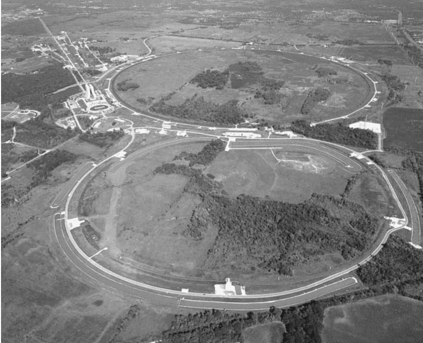
A 1999 aerial view of Fermilab shows the Main Injector (a proton synchrotron) in the foreground and Tevatron in the back. ( Fermilab Visual Media Services/Fred Ullrich )
