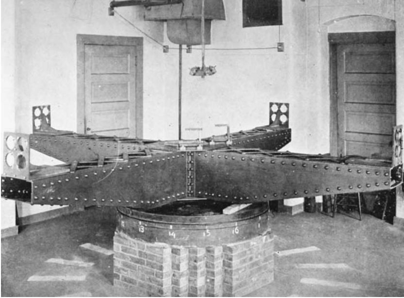
This interferometer, used by Edward Morley and a colleague, closely resembles the instrument with which Albert Michelson and Morley performed their experiments. ( AIP Emilio Segrè Visual Archives )
