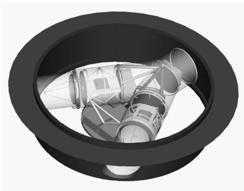
LISA spacecraft will have a Y-shaped structure; working together, the three vehicles form an extended interferometer. (NASA/JPL-Caltech)
