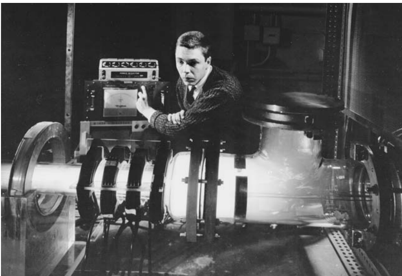
Accelerated by electromagnetic forces, the ions of this plasma move quickly. Plasmas can be used in this way to provide thrust for rockets. (NASA)
