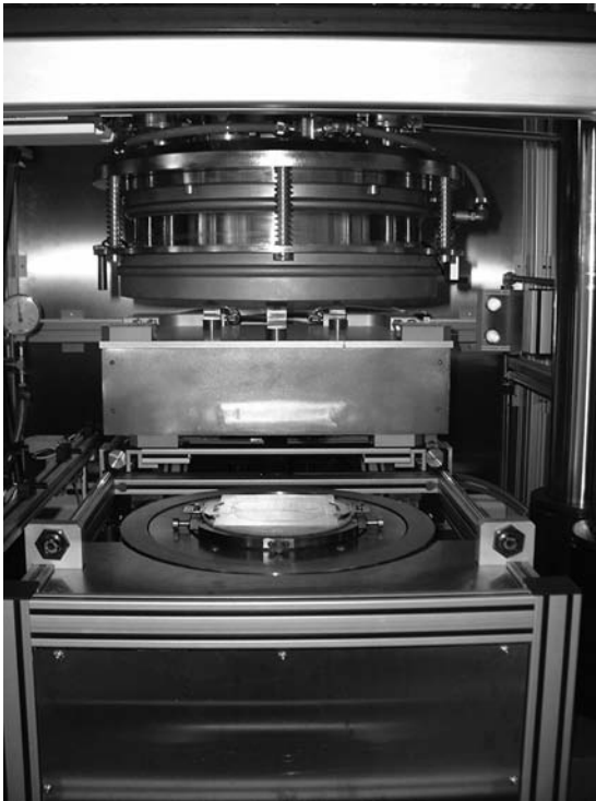
FIGURE 3.9 Jenoptik hot-embossing machine with microstructured polymer wafer. Reproduced courtesy of Application Center for Microtechnology (AMT), Jena, Germany ( www.amt-jena.de ).
