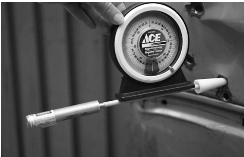
Figure 4.16 Using an angle gauge.
