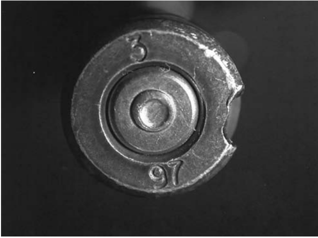
Figure 4.28 Deformed 7.62 × 39 cartridge case head.
