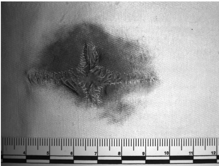
Figure 9.1 Long rifle (22-caliber) ammunition fired into cotton twill.
