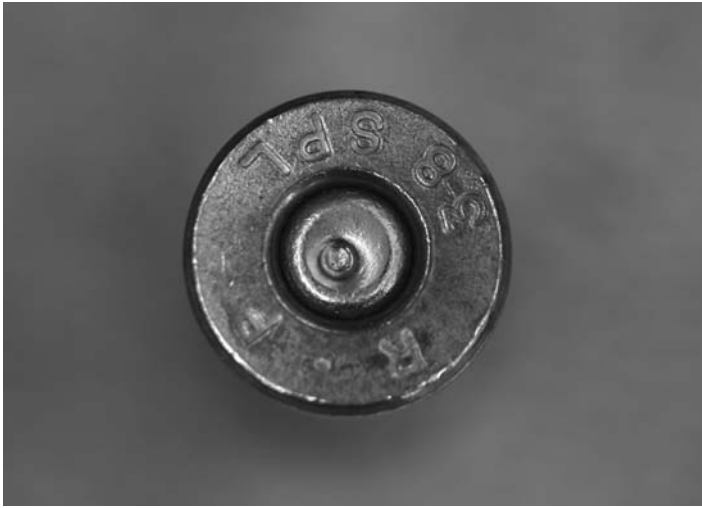
Figure 3.12 Center fire cartridge case.
