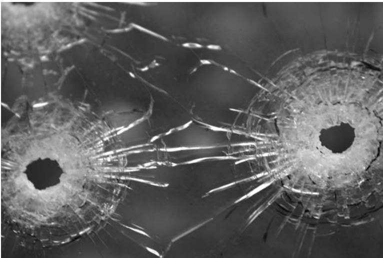
Figure 9.10 Radial and concentric fractures in safety plate glass.
