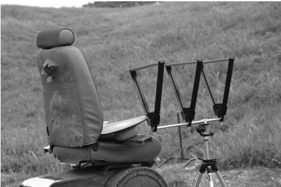
Figure 4.26 Use of chronograph to determine velocity of bullet after passing through seat back.
