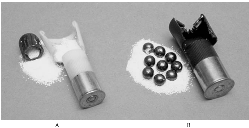
Figure 3.13 Shotgun slug (A) and size 00 buckshot (B).
