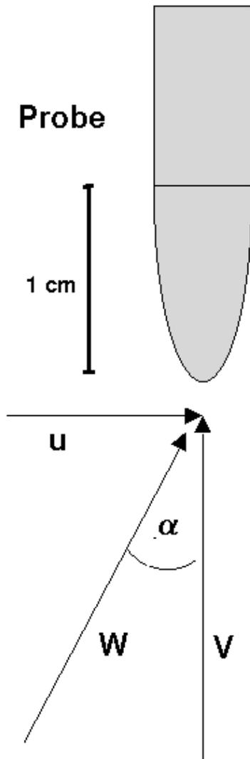
Geometry of the airfoil probe,  $\alpha$  is the angle of attack of the oncoming flow.
