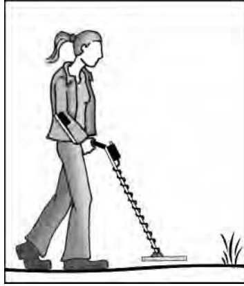
Figure 4.10 When using the metal detector, the coil should be held in front of the operator, parallel and as close to the ground as possible for maximum coverage and depth.
