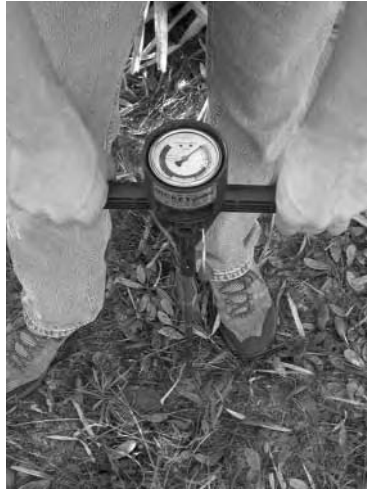
Figure 3.18 Use of a penetrometer probe with a gauge to show differences in soil compaction.
