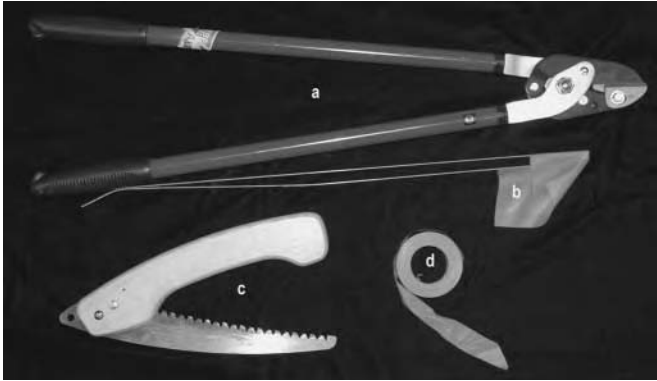
Figure 2.2 Equipment used during survey and clearing: (a) hand loppers; (b) survey flags; (c) hand saw; and (d) survey tape.
