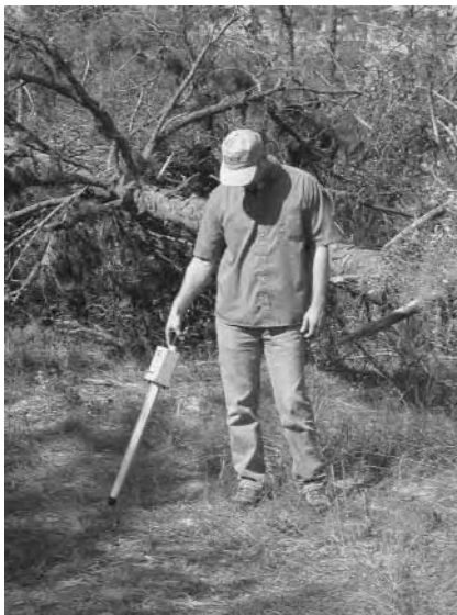
Figure 4.12 Author John Schultz demonstrating the use of a magnetic locator, which is swept from side to side while searching for buried metallic objects.
