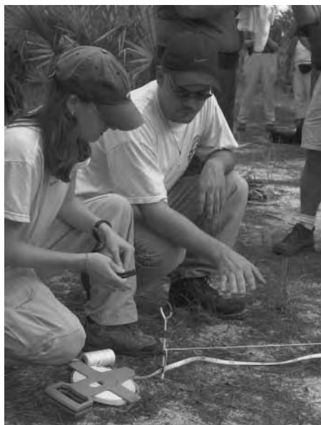
Figure 6.7 Author Sandra Wheeler assists a student in setting up a baseline using a compass and tape measure.
