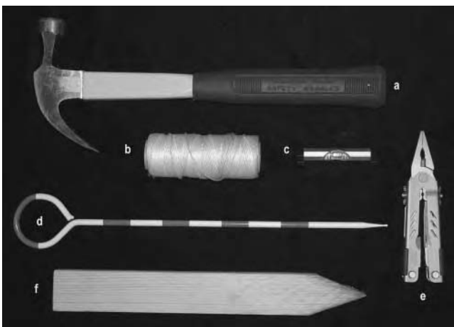
Figure 2.7 Equipment used for constructing grids: (a) metal hammer; (b) survey string; (c) line level; (d) chaining stake; (e) multipurpose tool; and (f) wooden stake.
