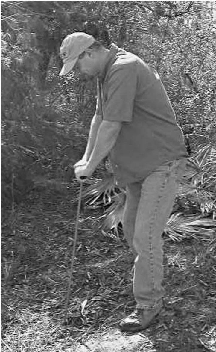
Figure 3.17 Author John Schultz demonstrates the use of a T-bar probe to detect differences in soil compaction in a depressed area.
