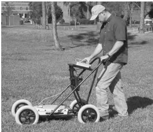
Figure 4.2 Author John Schultz demonstrating how the GPR is operated when using a survey cart with the 500-MHz antenna secured to the bottom of the cart.
