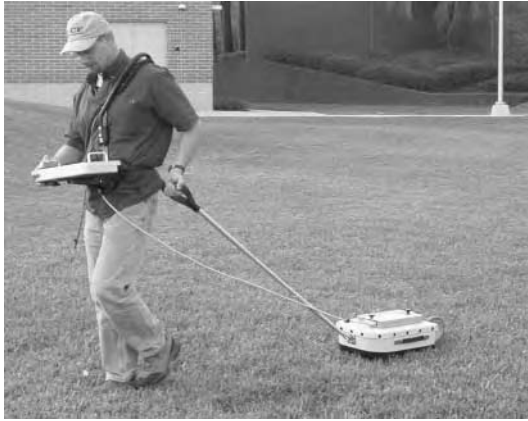
Figure 4.1 Author John Schultz demonstrating how the GPR is operated when one individual is pulling the 500-MHz antenna with the monitor secured to the body via a shoulder harness.
