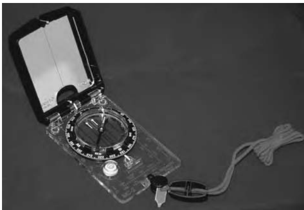
Figure 6.5 Example of a prismatic compass with a forward sight mirrored lid and base-plate with a rear sight.
