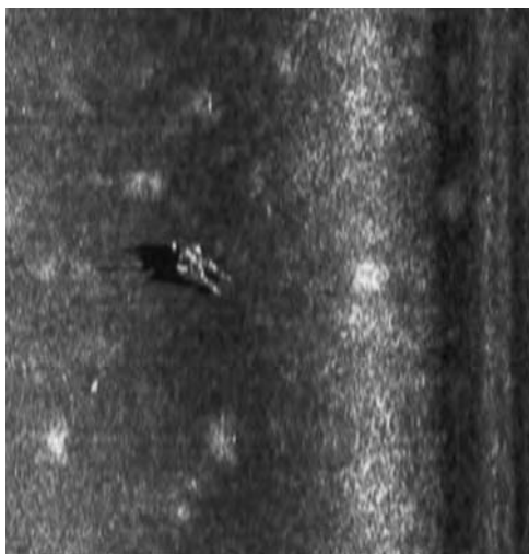
Figure 4.15 Side-scan sonar image of a drowned victim located on the bottom of a lake floor. (Photo courtesy of G. Ralston.)
