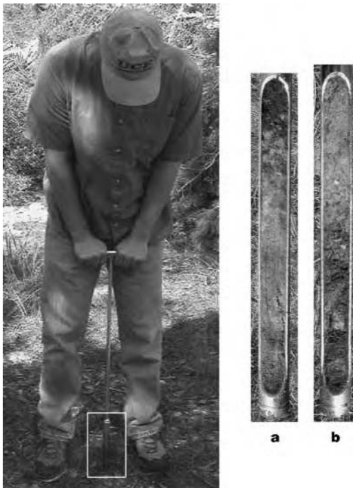
Figure 3.19 Author John Schultz demonstrates the use of a probe with soil corer to detect the presence of undisturbed or disturbed soil horizons: (a) soil core showing natural horizons; and (b) soil core showing mottled or mixed soil horizons.
