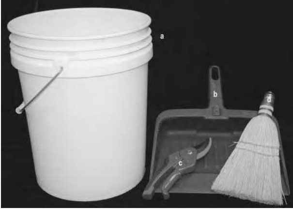
Figure 2.5 Equipment used for clearing and excavation: (a) spackle bucket; (b) plastic dustpan; (c) root clippers; and (d) whisk broom.
