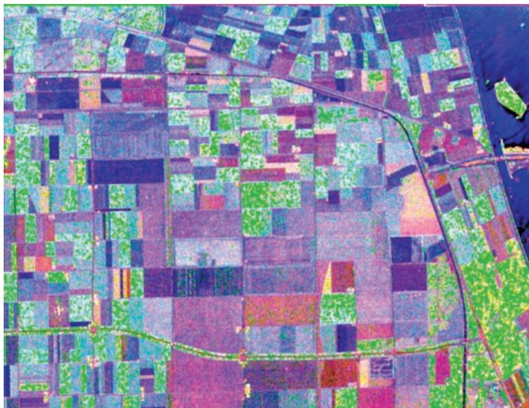
**Fig. 5.12** Freeman decomposition, Flevoland,  $L$  band.  $P_s$  (surface) in blue;  $P_v$  (volume) in green;  $P_d$  (double-bounce scattering) in red (POLoSAR-PRO result).
