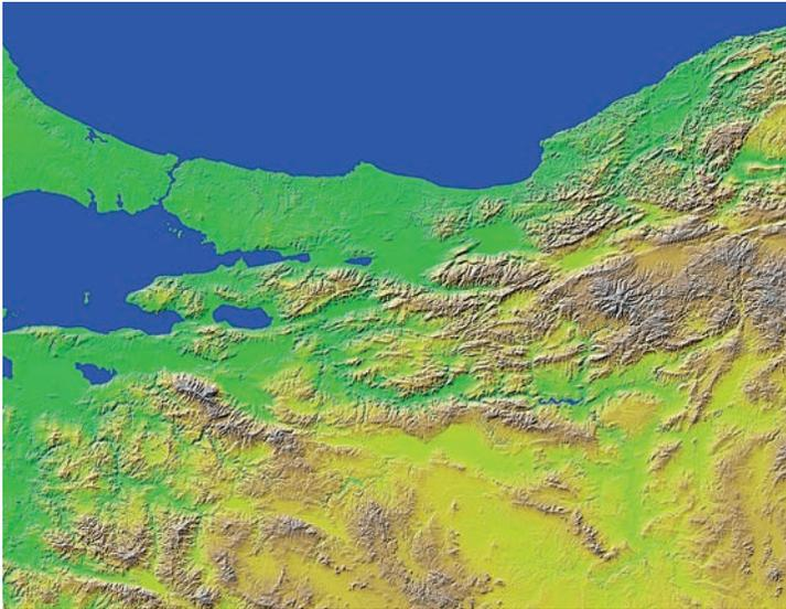
**Fig. 4.24** Example of low resolution SRTM DEM, Turkey. The horizontal posting is 90 m and the relative vertical resolution of the order of 10 m RMS.
