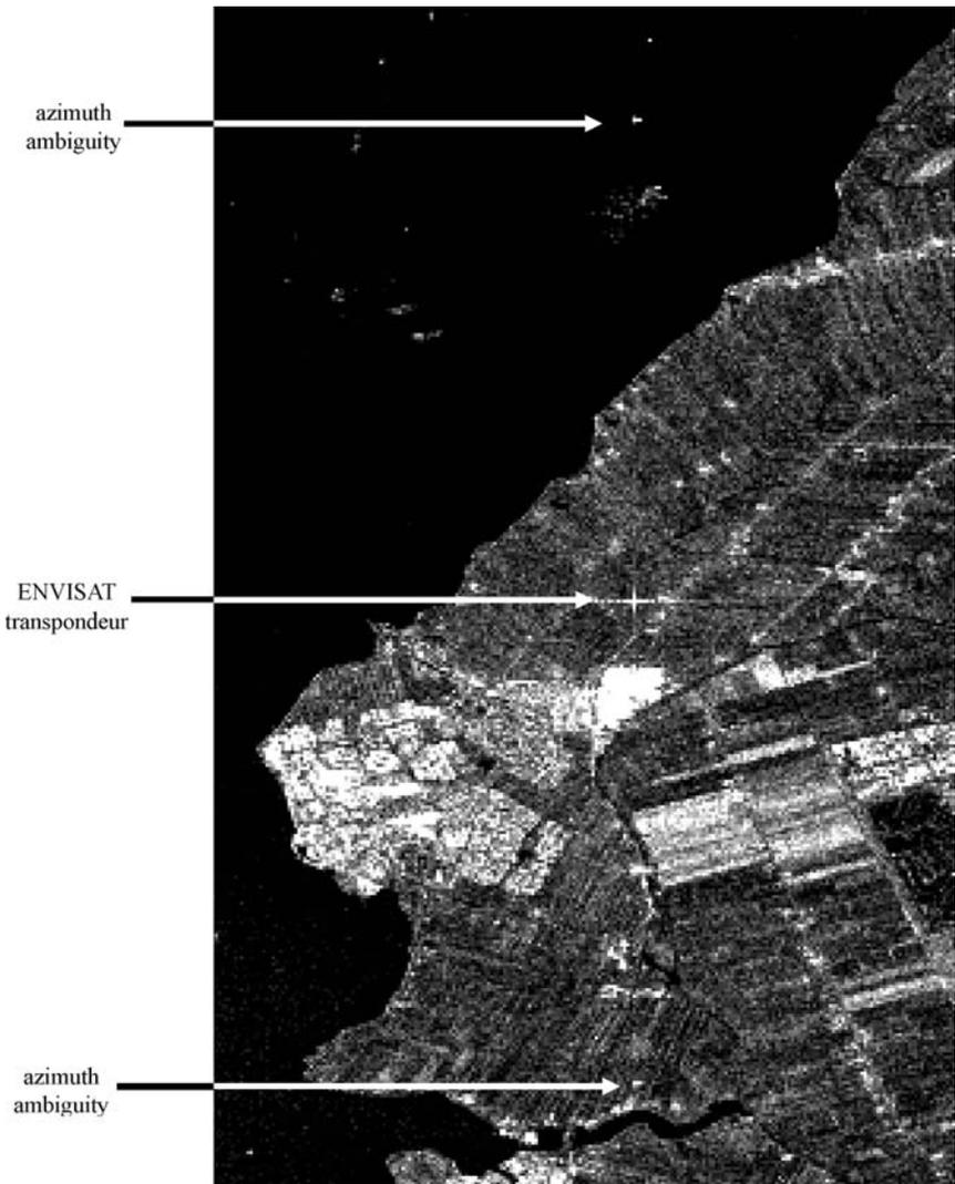
**Fig. 3.24** Radar signature of a transponder and its two main azimuth ambiguities (ASAR/ENVISAT S4 *HH*, of Edam, Holland, Oct. 02). Copyright ESA.
