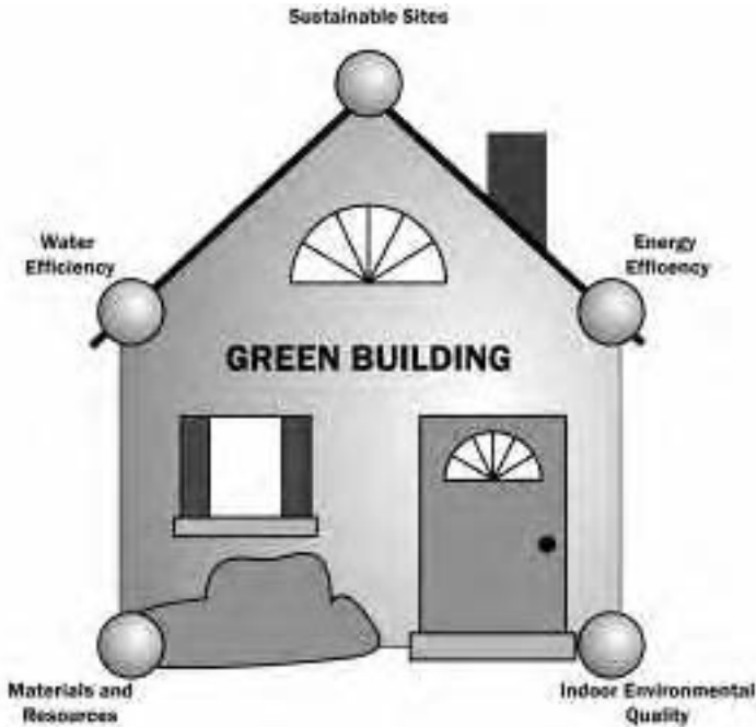
The “house” of green building showing the five major categories of concern.
