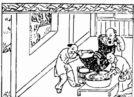
Series of woodcuts showing early Chinese ink production. At this stage the mixture included lamp-black, glue, and water. From Kamisuki Chohoki's A Handy Guide to Papermaking .
