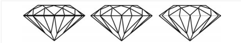
Shown here are diamonds with (in order) too large, perfect, and too small girdle.
