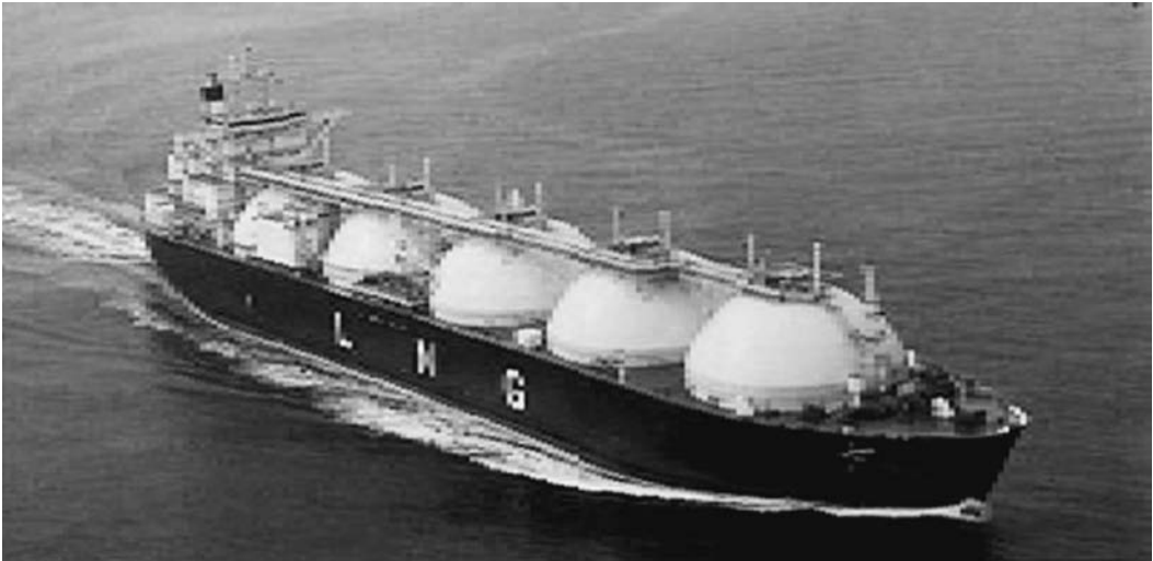
FIGURE 10.1 Moss spherical tank LNG carrier.
