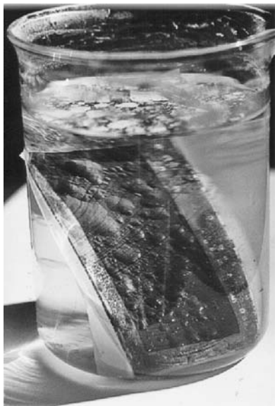
FIGURE 1.13 Steel sample coated with a polyaniline primer and an epoxy topcoat after a 3-yr immersion in saltwater—note the absence of corrosion products in the test solution.
