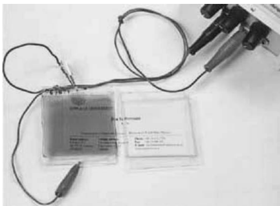
FIGURE 1.8 Example of electrochromic device based on polypyrrole-coated glass.
