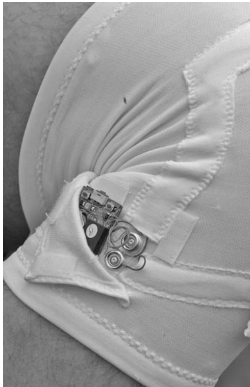
FIGURE 1.19 Example of fabric strain gauge for determining knee flexion; such devices can be used in sports training, biomechanics studies, and rehabilitation.
