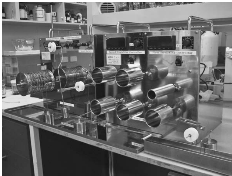
FIGURE 7.9 The customized wet-spinning apparatus at the Intelligent Polymer Research Institute, University of Wollongong.
