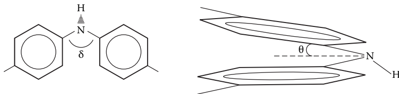
FIGURE 4.3 Definition of the chain angles \delta (bond angle ring-amine N-ring) and \theta (ring torsional twist).
