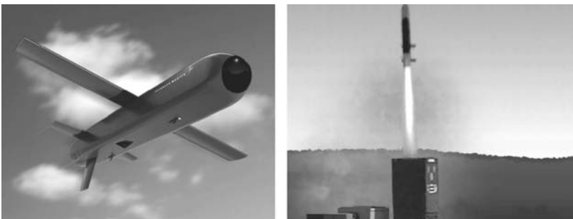
FIGURE 2.23 Lockheed-Martin NLOS-LAM: left , flight configuration; right , munitions being launched. (Courtesy of Lockheed-Martin.)
