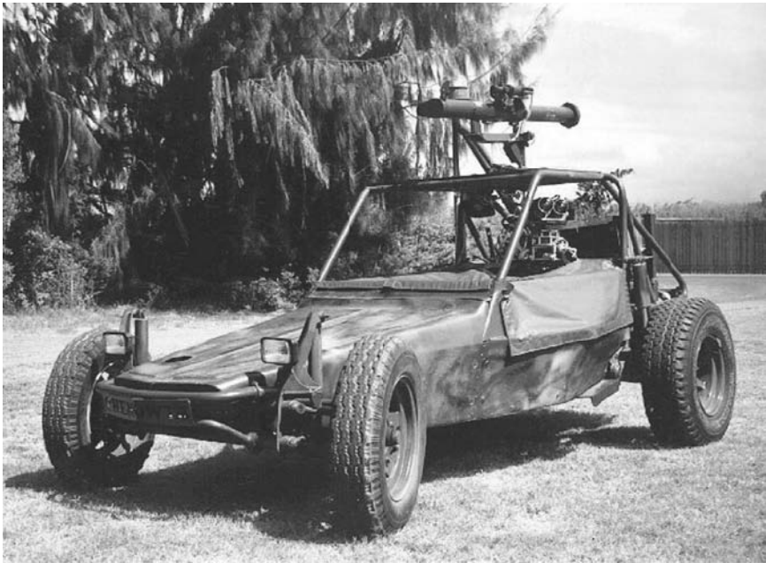
FIGURE 2.12 Teleoperated dune buggy (1985) equipped with an antiarmor rocket launcher. (Courtesy Space and Naval Warfare Systems Center Pacific.)
