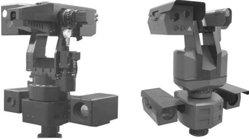
FIGURE 2.3 Samsung Techwin intelligent surveillance and security guard robot: left , prototype; right , newer model SGR-A1. (Courtesy of Samsung Techwin.)
