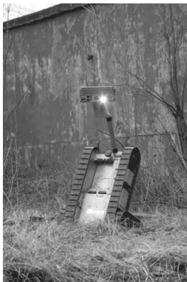
FIGURE 11.7 An iRobot Packbot 500 equipped with a Red Owl Sniper Detection Kit. (Courtesy of iRobot.)
