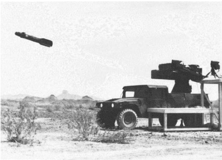
FIGURE 2.13 GATERS UGV (1989) launching a Hellfire missile by remote command from an operator located several kilometers away. (Courtesy Space and Naval Warfare Systems Center Pacific.)
