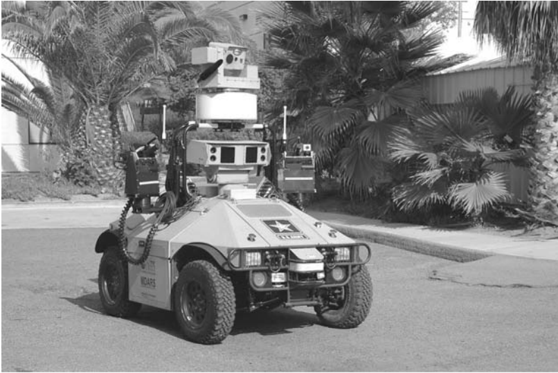
FIGURE 2.14 MDARS with PUV equipped with less-than-lethal weapons systems. (Courtesy Space and Naval Warfare Systems Center Pacific.)
