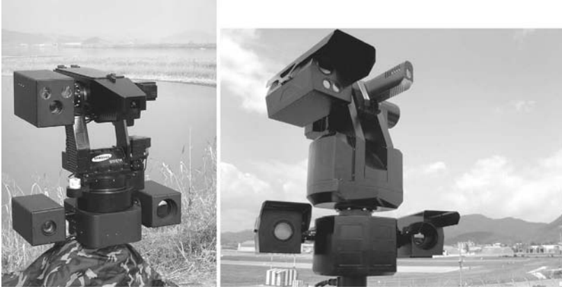
FIGURE 11.3 Left , Samsung intelligent surveillance and security guard robot prototype; right , newer-model SGR-A1. (Courtesy of Samsung Techwin.)
