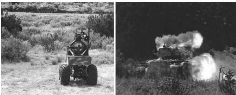
FIGURE 2.10 Sandia’s Fire Ant robot: left , deployed by the roadside in wait for a target; right , the results of the Fire Ant’s weapons discharge, destroying a tank. (Courtesy Sandia National Laboratories.)
