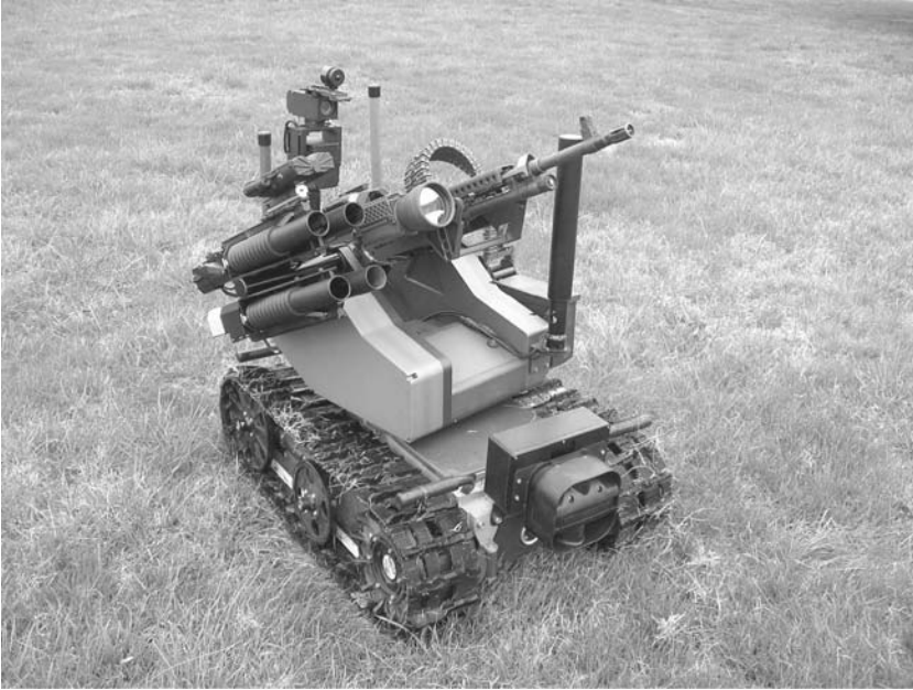
FIGURE 2.6 MAARS robot. Like SWORDS, it is not autonomous. (Courtesy of QinetiQ North America/Foster-Miller.)
