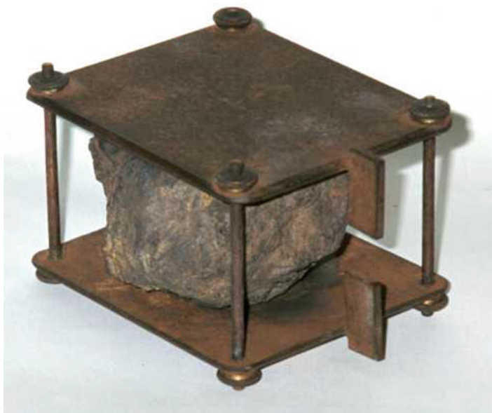
Fig. 4.2 A lodestone sandwiched, as if it might inexplicably fly away, between two iron plates. A strong magnetic field is established between the two vertical vanes (Image courtesy of Westminster College, Pennsylvania: http://physics.kenyon.edu/EarlyApparatus/index.html )
