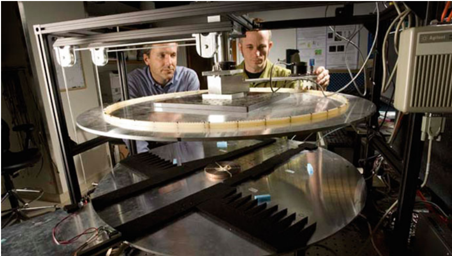
Fig. 3.35 Steve Cummer ( left ) and David Schurig ( right ) making adjustments to the acoustic cloak testbed. A microwave invisibility cloak (to be described in Chap. 5 – but recall Fig. 3) can be seen on the lower disk of the testbed (Image courtesy of Duke University)
