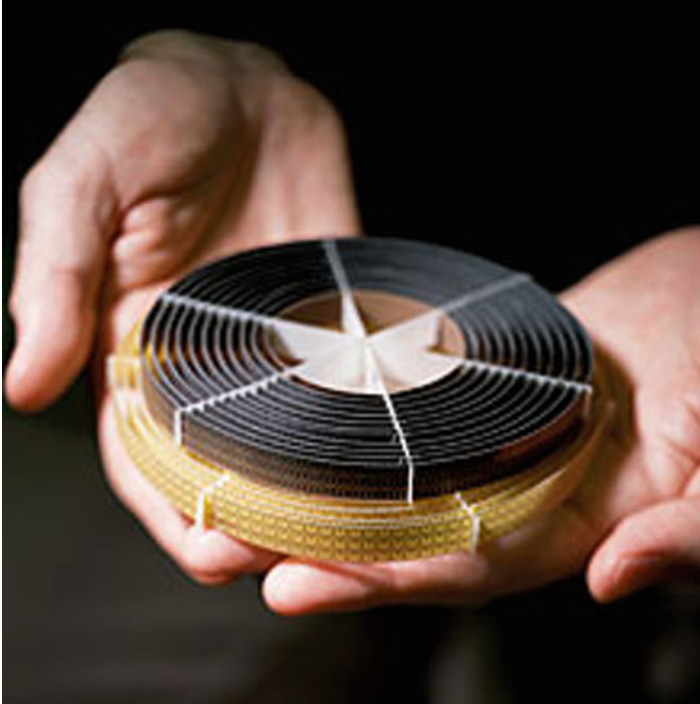
Fig. 3 Two of the very first experimental cloaking devices. These disks can mask from view (at microwave wavelengths) any object placed within their central core (Image courtesy of D. Smith, Duke University)
