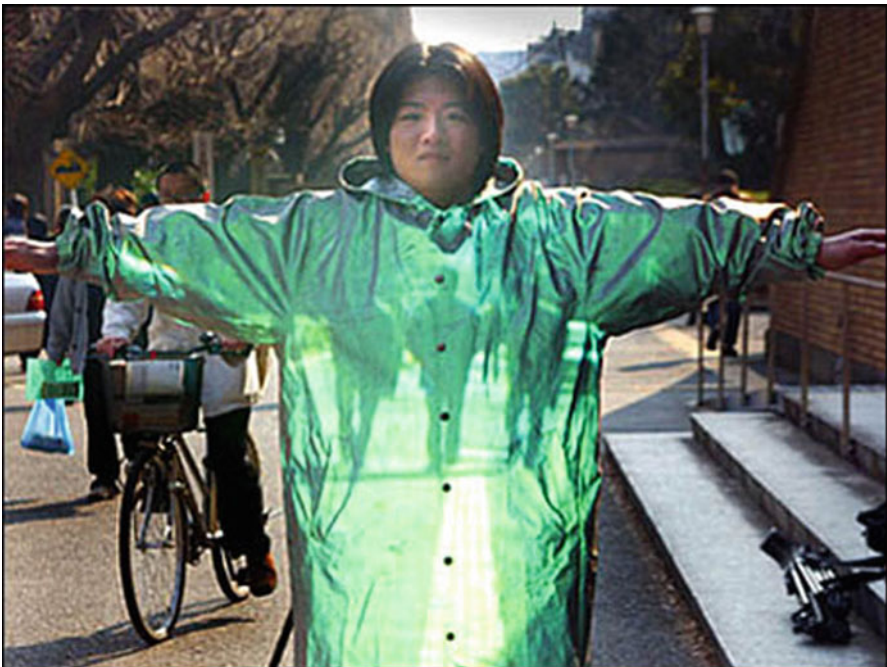
Fig. 3.4 A real-life example of invisibility cloaking. The view occulted by the central figure is projected seamlessly onto the front of the cloak, making the wearer appear (partially) invisible (Image courtesy of Tachi Labs, The University of Tokyo)
