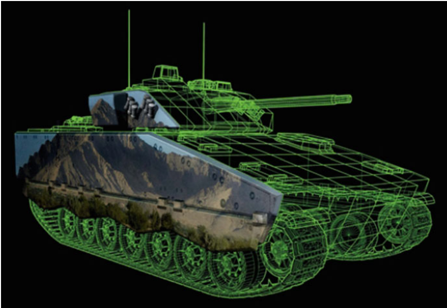
Fig. 3.6 The adaptive E-ink camouflage developed by BEA Systems updates the image portrayed on each side of a tank, making it blend into the background (Image courtesy of BEA)
