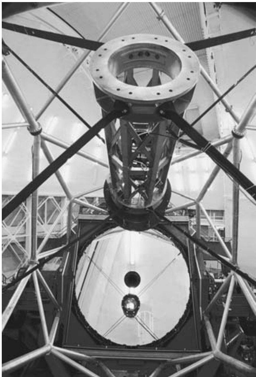
Figure 2.5. The completed and operational 8.1-m-diameter Gemini North telescope is shown here. Notice the minimal skeletal supporting structure for the primary and secondary mirrors. The primary mirror has a diameter of 8.1 m, and the secondary mirror can be seen in reflection. Courtesy of National Optical Astronomy Observatory.
