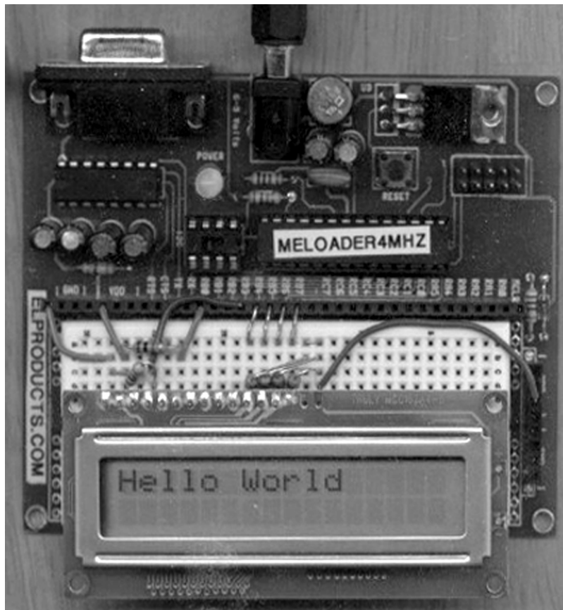
Figure 7-2: View of the complete LCD module circuit board.
