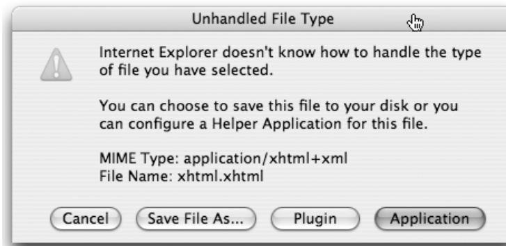
Figure A-2. Internet Explorer tries to download the file instead of displaying it.
