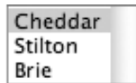
Figure 4-19. A list menu, created with a <select> with an attribute of multiple
