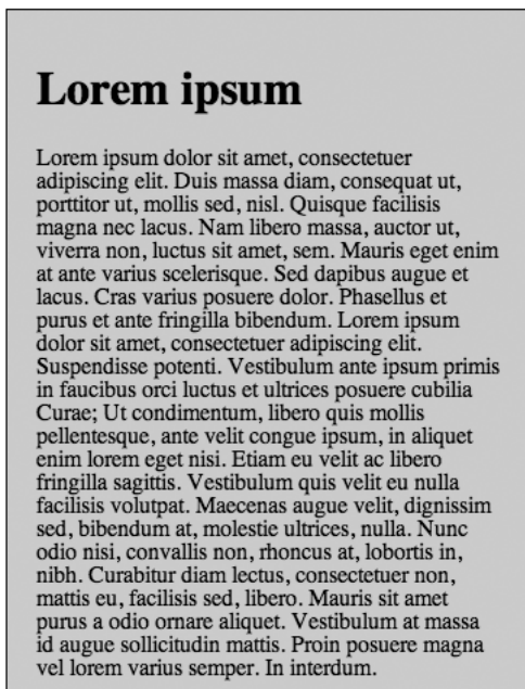
Figure 6-7. The <html> root element has been styled, which causes the <body> element to be treated as a regular <div> .
