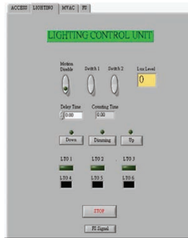
Figure 4. Lighting control panel
