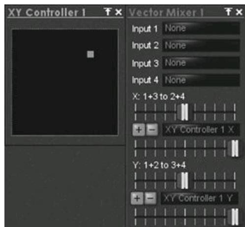
Figure 6.30 The XY Pad in VAZ Modular hooked up to a Vector Mixer.
