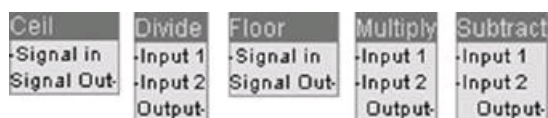
Figure 7.21 The mathematical function units in SynthEdit. From left to right: Ceiling, Divide, Floor, Multiply, and Subtract.
