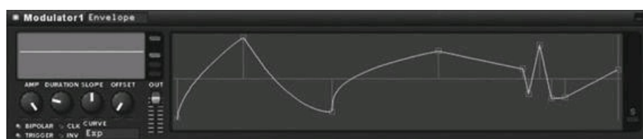
Figure 6.12 The Envelope module in KarmaFX Synth Modular in a multi-stage envelope with bipolar capability.
