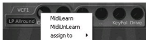
Figure 6.31 MIDI Learn and MIDI UnLearn in Zebra 2. You will also notice the Assign To submenu, which can be used to assign the knob's function to the XY pad.
