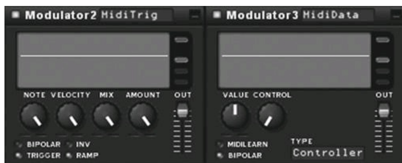
Figure 7.13 MIDITrig and MIDIData modules in KarmaFX Synth Modular.
