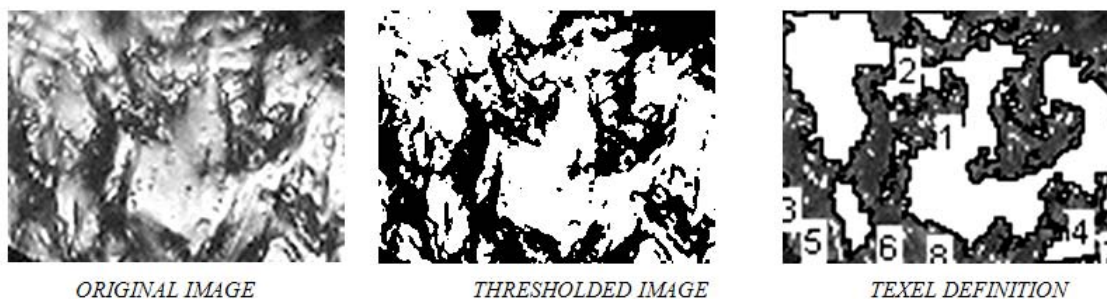
Figure 7.4. Determining use-wear texels using luminance thresholds. In this example, 120 grey levels have been selected as threshold.
