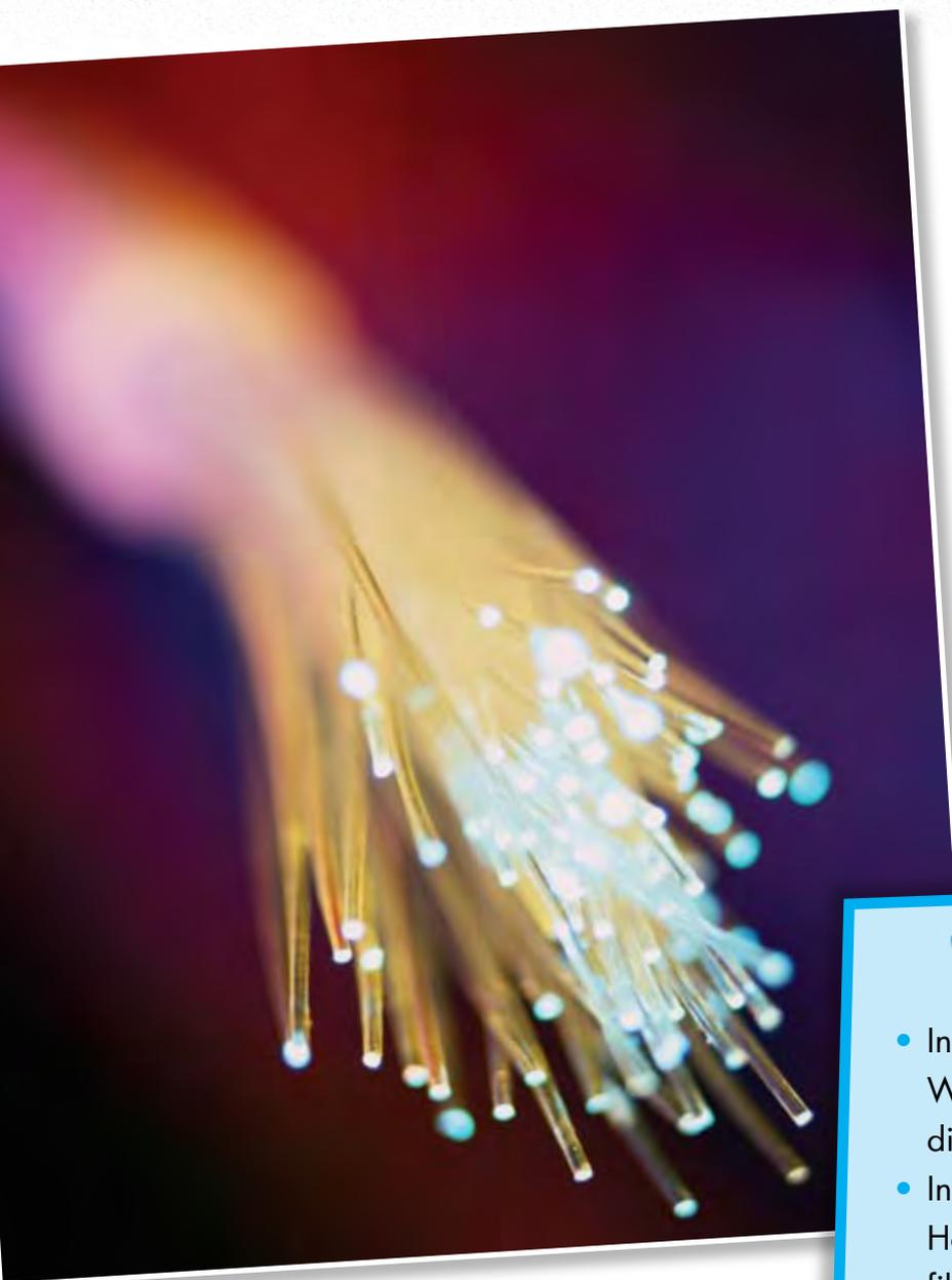
Optical fibers are thin filaments of glass that are used as communication cables. They use light beams to transmit audio, video, and data. They work on the principle of total internal reflection. They have enormous data carrying capacity at low-cost. In 1930 Heinrich Lamm, a German student, became the first person to use optical fibers to carry an image.
