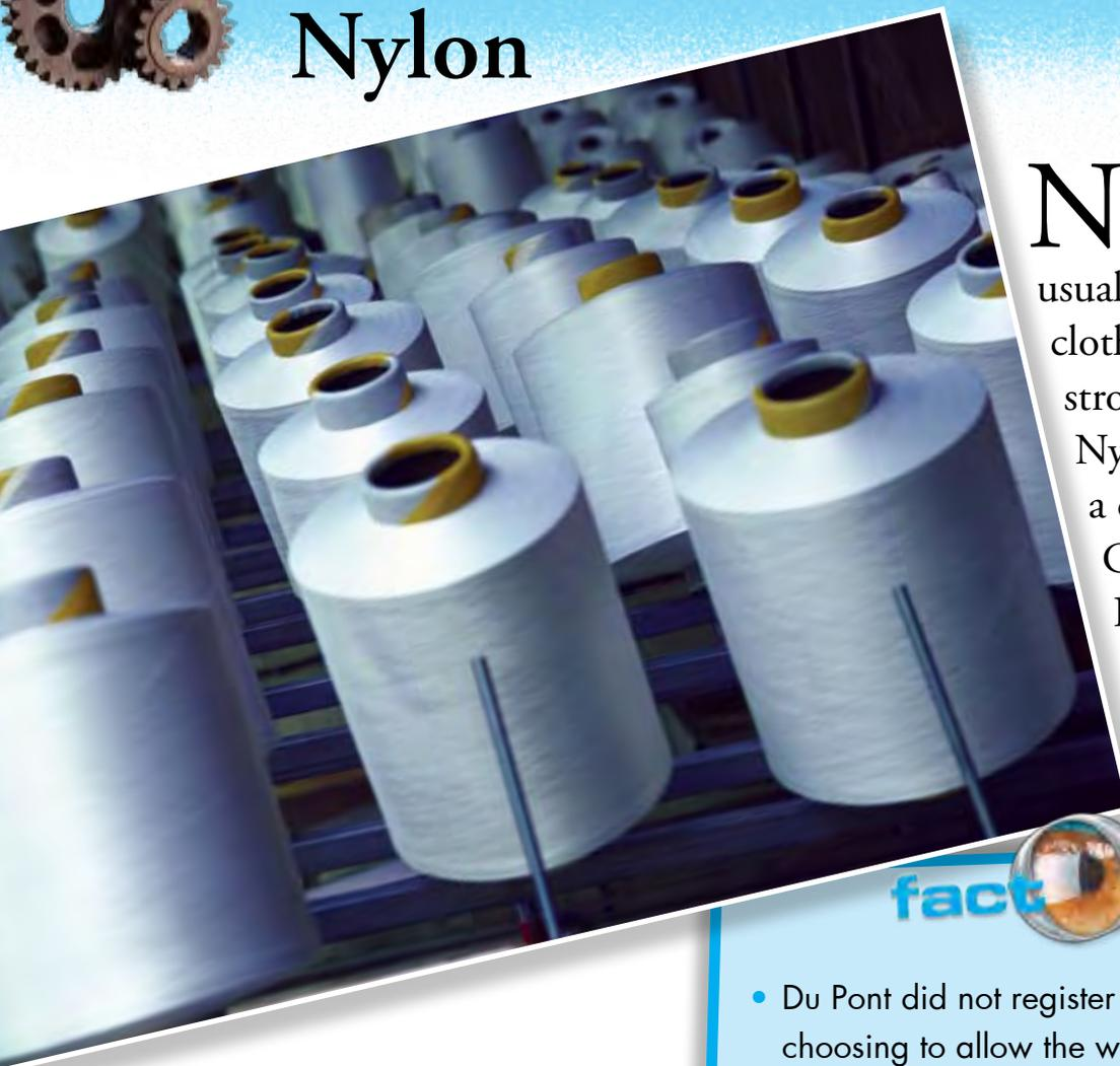
Nylon is a manmade synthetic material usually used for making clothes. It is an extremely strong, synthetic fiber. Nylon was invented by a chemist, Dr. Wallace Carothers, at the Du Pont Company in 1935. Du Pont named this fiber "nylon."
