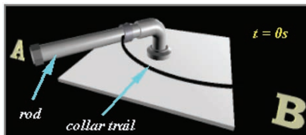
Figure 11. Linear motion of the rod and collar rotating about y-axis ( t = 0 s)
