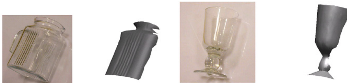
Figure 8. From left to right: Glass container and its 3D representation obtained from SFH, Glass and its 3D representation obtained from SFH
