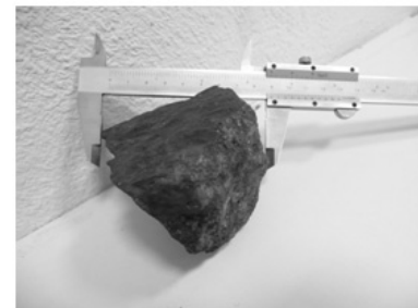
Measuring maximum height with a caliper.
