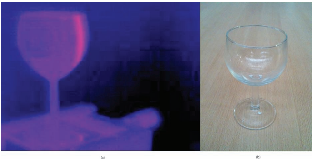
Figure 7 (a) Images of a heat pattern released in the case of a glass; (b) scanned using the Scanning from heating: Line configuration (Meriaudeau, 2010)
