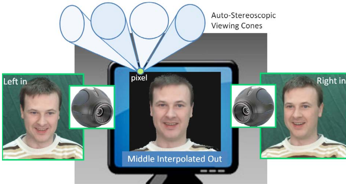
Figure 1. Interpolation of Left/Right camera views into a rendered virtual viewpoint for eye-gaze correction in video teleconferencing (bottom), possibly augmented with auto-stereoscopic 3D displays where each pixel projects multi-directional viewing cones from which two are captured by the viewer's eyes (top)
