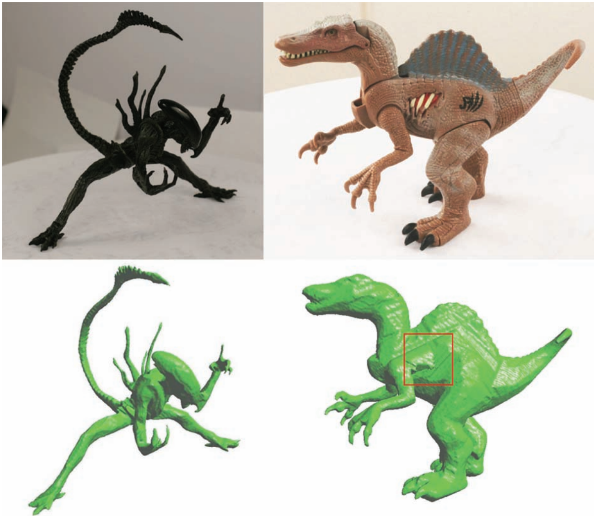
Figure 1. The visual hull of a toy alien model (left) and a toy dinosaur model (right)
