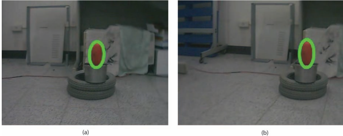
Figure 4. Position deviations between the robot and the fire and viewpoint from the robot's first and second camera after applying the visual servoing rules
