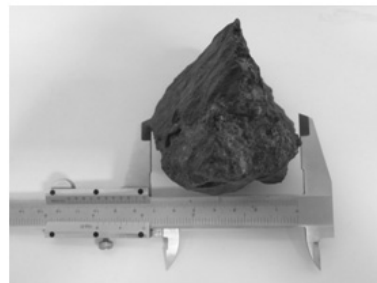
Measuring maximum width with a caliper.
