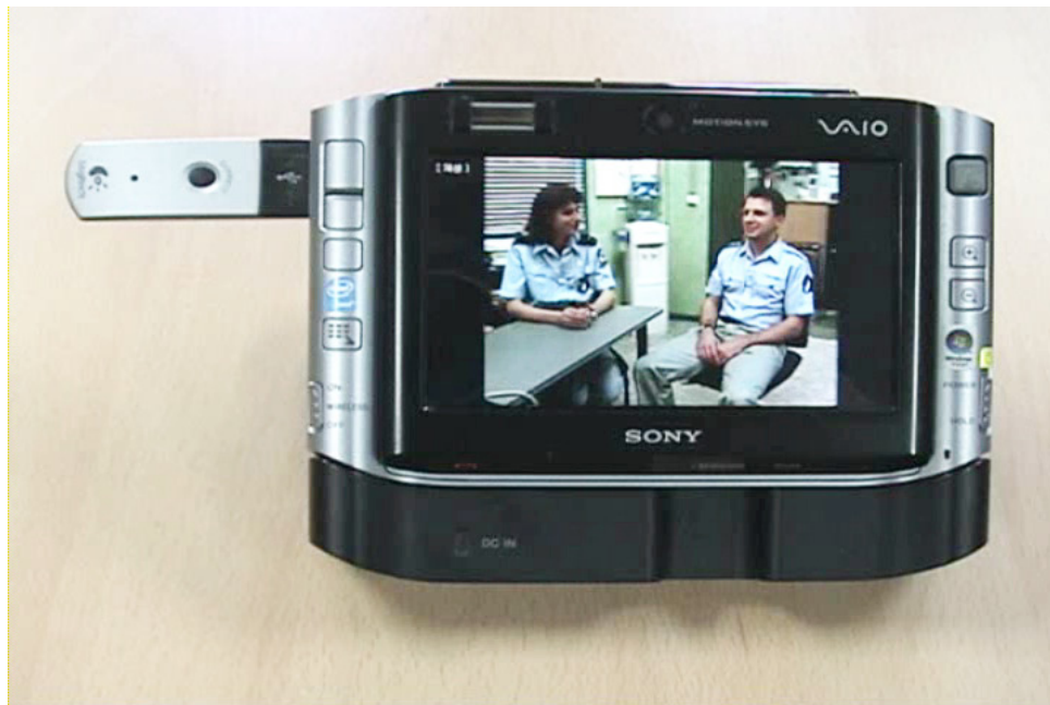
Figure 7. Our 3D DMB player: the special parallax barrier is affixed to the display of the SONY VAIO VGN-UX17LP for viewing 3D auto-stereoscopic images
