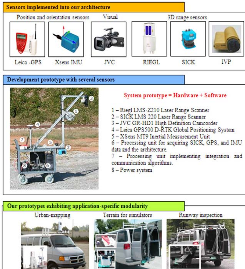
Figure 6. The sensor architecture lends to different levels of modularity with large-scale mapping. After testing a development prototype on a push cart (middle row), we have improved towards application-specific professional packaging (bottom row).
