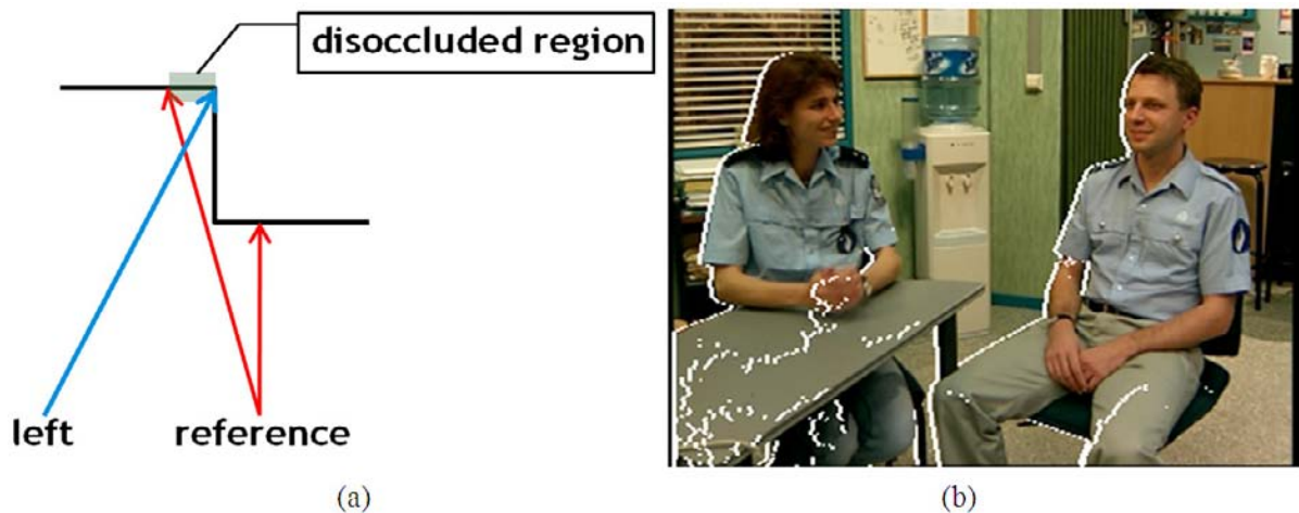
Figure 5. Holes caused by disoccluded regions. (a) Cause of disoccluded regions. (b) Virtual left view of 'Ballet' sequence (white pixels are the disoccluded regions).
