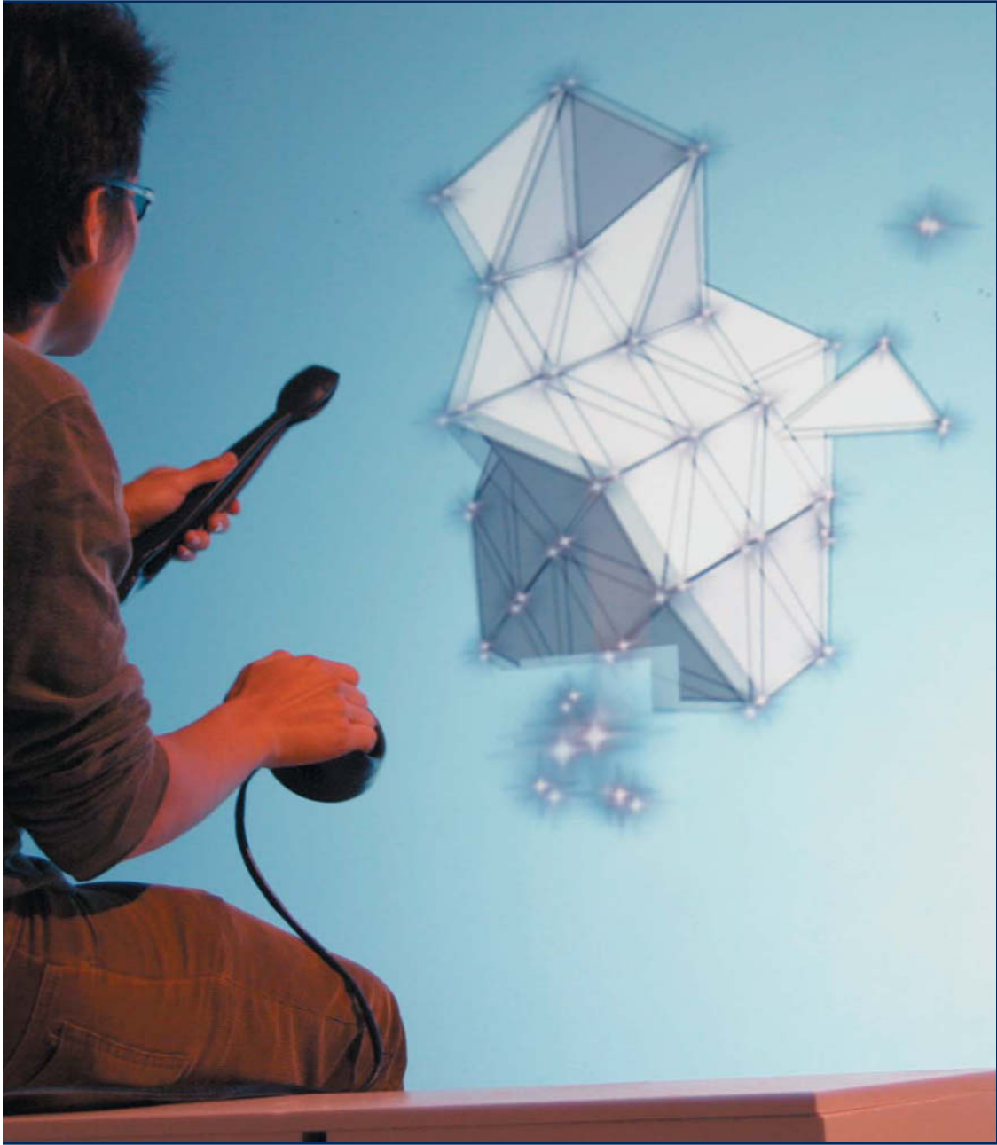
Crystal Method by Steven Schkolne showing shape drawn in space that can be grabbed and rotated using sensing tool. Courtesy of Nano Creative Group.
