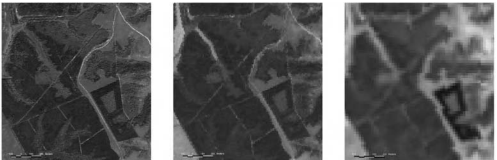
Fig. 4.2. Different resolution of remotely sensed images for the same area. Left: Quick Bird image (pixel of 2.8 m). Centre: SPOT XS (pixel of 10 m). Right: Landsat 7 ETM+ (pixel of 30 m). All images are compositions of RGB 432 in grey-scale palette.
