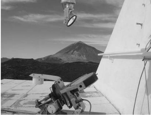
**Figure 7.2.** At the Observatorio del Teide on Tenerife – the Birmingham Mark I instrument is housed in the pyramid building shown on the right, and fed sunlight by a system of mirrors (a cœlostat). Pico de Teide looms large in the background. Picture courtesy of S.J. Hale.
