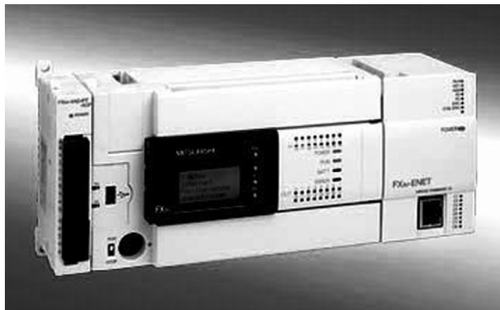
Figure 1.13: Mitsubishi Compact PLC: MELSEC FX3U. (By permission of Mitsubishi Electric Europe.)
