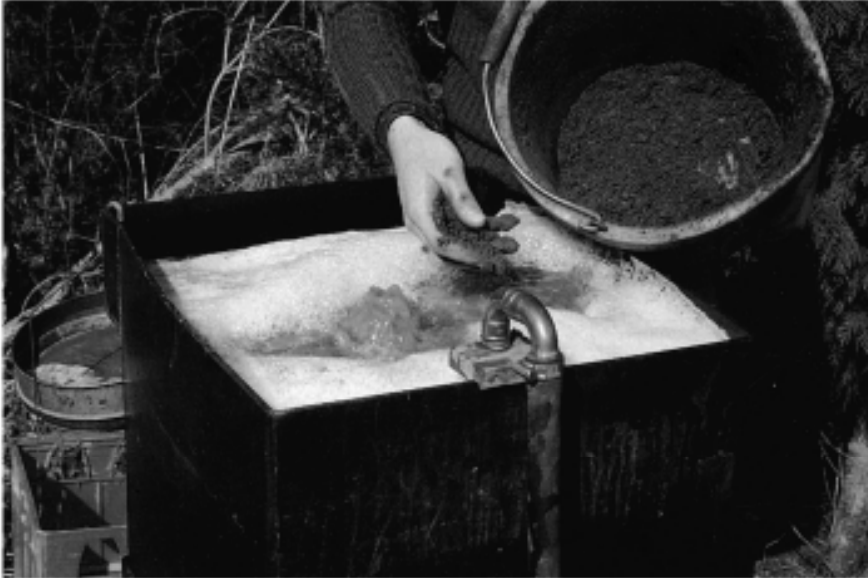
Figure 5.17 Recovering carbonized material with a froth flotation unit.
