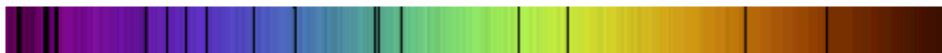
Fig. 1.14. White light from a star when passed through a glass prism is spread into a spectrum of colors. Dark lines correspond to the absorption of light of precise color by atoms in the star’s atmosphere. By comparing them with the lines of known atoms in the laboratory, the type of atoms present in the star’s atmosphere can be identified. If the lines in the star’s spectrum are Doppler-shifted by the star’s motion, a measurement of the shift reveals the speed at which the star is approaching or receding from the Earth.
