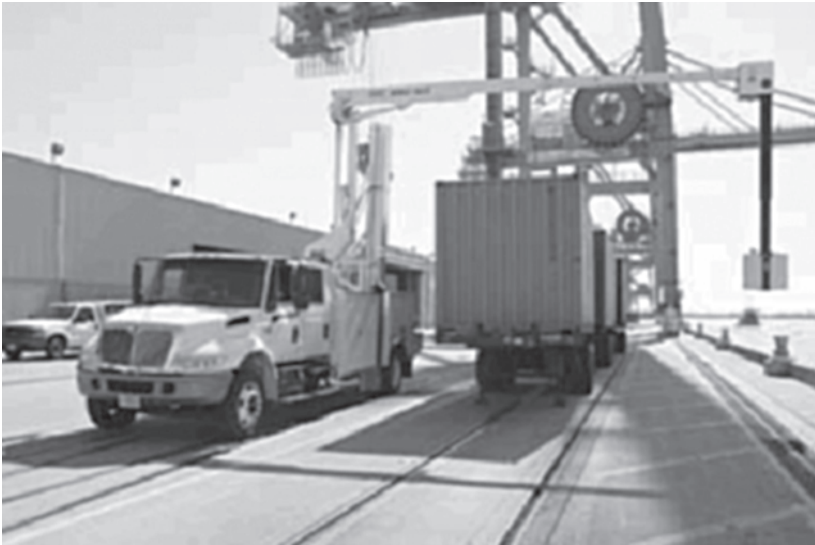
Figure 2.1. Advance applied X-ray technology allows Customs officers to see inside entire seaport containers. (X-ray container exam compliments of www.cbp.gov photo gallery.)
