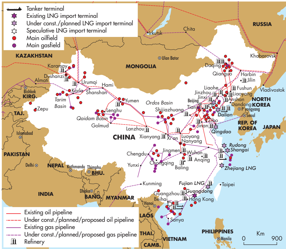
Figure 10.1: China's Oil and Gas Resources and Supply Infrastructure
