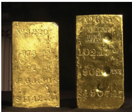
▲ FIGURE 4.15 The chemical inertness of gold. Two, stamped, weighed, and priced (in the 1800's) gold bars recently recovered from a steamship that sank off the coast of Central America in 1857.
