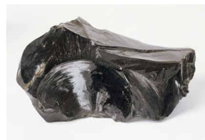
Obsidian (typically \text{KAlSi}_3\text{O}_8 ), an amorphous solid
