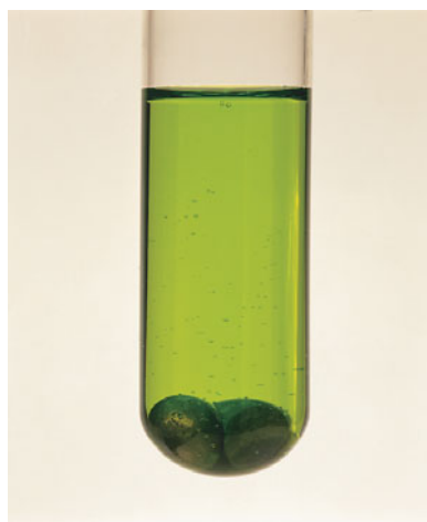
Nickel reacts with hydrochloric acid, forming \text{NiCl}_2(aq) and \text{H}_2(g) . The solution is of \text{NiCl}_2 , not Ni metal
