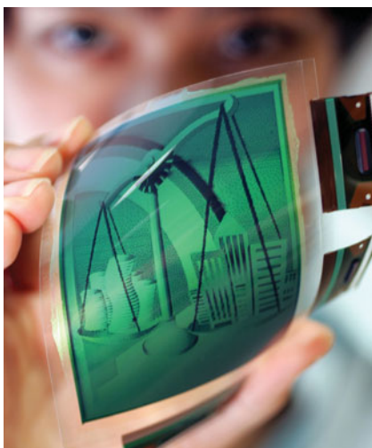
▲ FIGURE 11.35 Electronic paper (e-paper) based on cholesteric liquid crystal technology.
