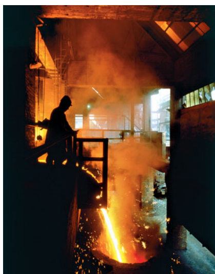
▲ FIGURE 6.5 Color and temperature. The color and intensity of the light emitted by a hot object, such as this pour of molten steel, depend on the temperature of the object.
