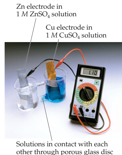
▲ FIGURE 20.4 A Cu-Zn voltaic cell based on the reaction in Equation 20.7.
