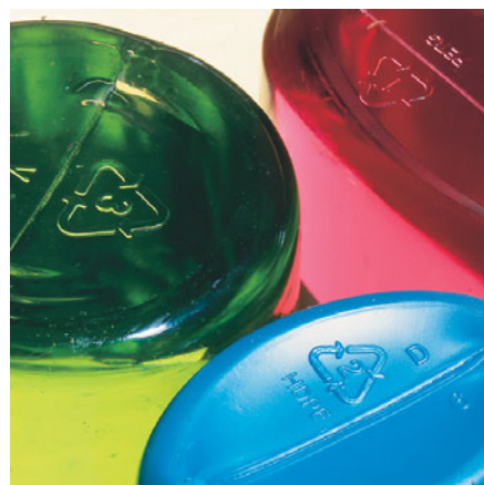
▲ FIGURE 12.36 Recycling symbols. Most plastic containers manufactured today carry a recycling symbol indicating the type of polymer used to make the container and the polymer's suitability for recycling.
