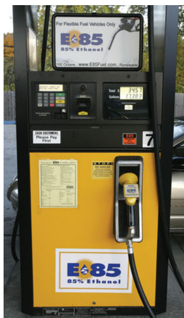
◀ FIGURE 1.20 A gasoline pump that dispenses E85, a mixture of 85% ethanol and 15% gasoline.
