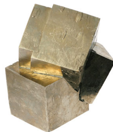
Iron pyrite ( \text{FeS}_2 ), a crystalline solid
