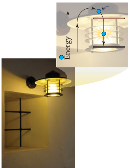
▲ FIGURE 7.22 The characteristic yellow light in a sodium lamp is the result of electrons in the high-energy 3p orbital falling back to the lower-energy 3s orbital. The energy gap corresponds to the energy of yellow light.
