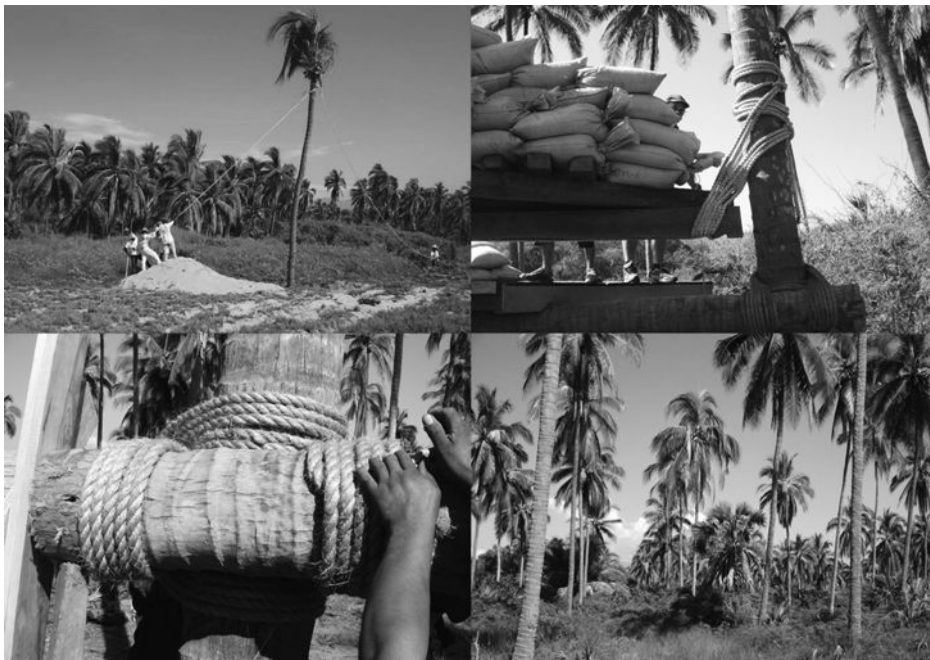
Figure 7-6 These images show tests used to evaluate the ability of transplanted palms (technically a grass) to reestablish themselves such that they are able to hold the living matrix of sand and soil together (they did) and the process of structural testing to use them as “living columns” for casitas at Playa Viva, an ecoresort in Juluchuca, Mexico. Images by David Leventhal, Playa Viva, http://www.PlayaViva.com .
