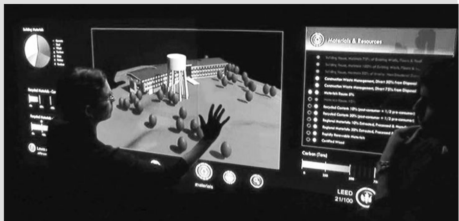
Figure 6-1 Interactive multi-touch screen built by Perceptive Pixel to demonstrate the future of integrating building information modeling (BIM), building form, energy modeling, and LEED software to allow users near-real-time feedback on building performance impacts of design options (presented at the Opening Plenary of U.S. Green Building Council's annual Greenbuild, November 2007). Image reproduced with the permission of Autodesk, Inc. ©2008. All Rights Reserved.
