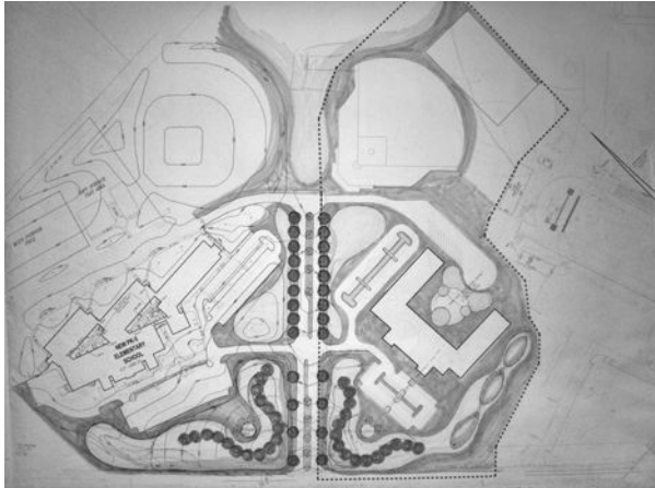
Figure 7-4 This sketch presented by the landscape architect at a Miami Trace Middle School team workshop depicts large wetland and rain garden areas that collect and infiltrate rainwater, thereby eliminating a much more costly system of stormwater detention and conveyance for the new middle school (located to the right of the road). The concept was generated at an earlier team workshop (see Figure 7-5). Image courtesy of Marcus Sheffer.
