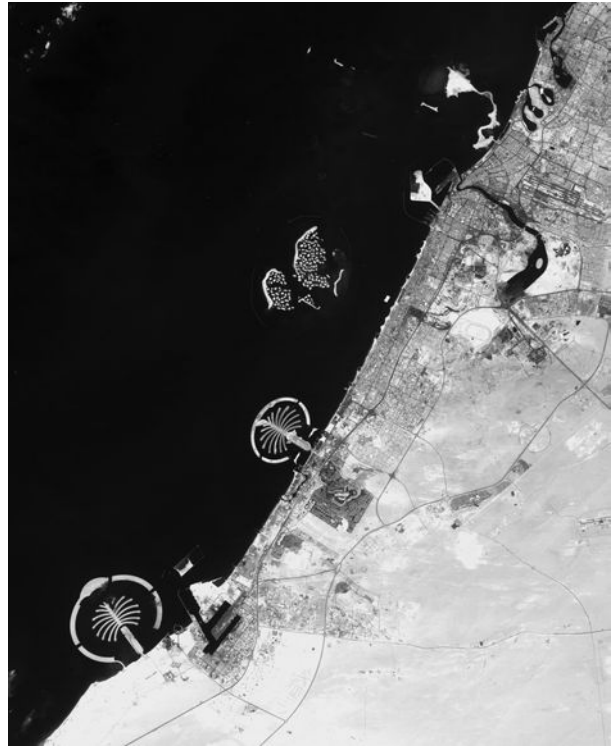
Figure 3-1 The Dubai Palms and World projects consist of artificially built islands in the Persian Gulf constructed for high-end commercial and residential development. In this image, we see (from the bottom left) Palm Jebel Ali, Palm Jumeirah, the World (configured to depict a world map when viewed from the sky), and Palm Deira, which is in the early stages. Although environmental concerns mandated that no concrete be used for these monumental engineering projects, dredging of the sand needed for the underlying structure of the islands depleted the local sea bed, so sand from the northern Persian Gulf had to be imported. Image courtesy of NASA.
