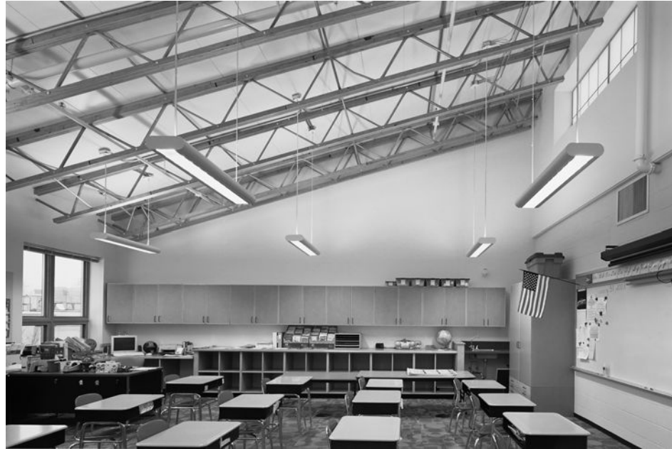
Figure 2-3 A classroom at Clearview Elementary School in Hanover, Pennsylvania, exhibits excellent bilateral daylighting, allowing daylight to enter from both the north and the south. Copyright © Jim Schafer.
