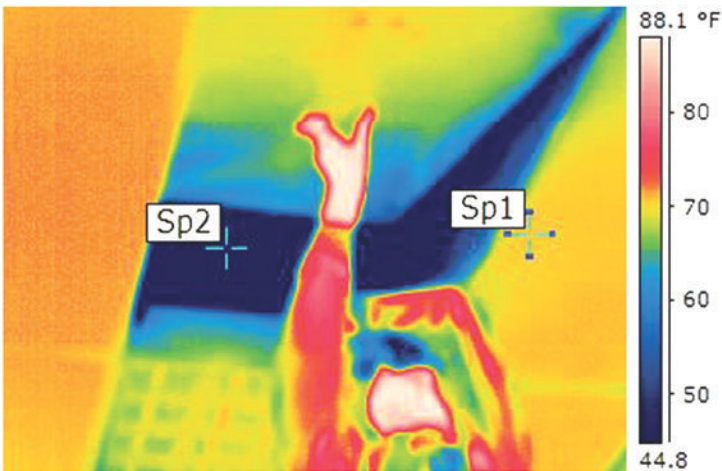
Figure C-7 Poor construction practices often cause thermal envelope failure; for example, the gaps depicted in this image will allow air to pass freely between the interior and exterior. Such envelope failures can be avoided by including envelope commissioning in a project's scope of commissioning services. Image courtesy of Brian Toevs.
