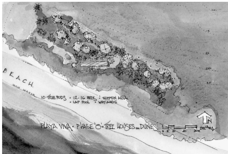
Figure 4-4 This site plan rendering for the casitas at Playa Viva resulted from examining large-scale bioregional patterns and relationships beyond the project property, resulting in a “tree-house structures” concept that minimally disturbs the site’s natural water flows and helps restore the ecosystem of the damaged coastal sand dunes. Design by Regenesis and Ayrie Cunliffe. Drawing by Ayrie Cunliffe. Image courtesy of David Leventhal, Playa Viva, http://www.PlayaViva.com .
