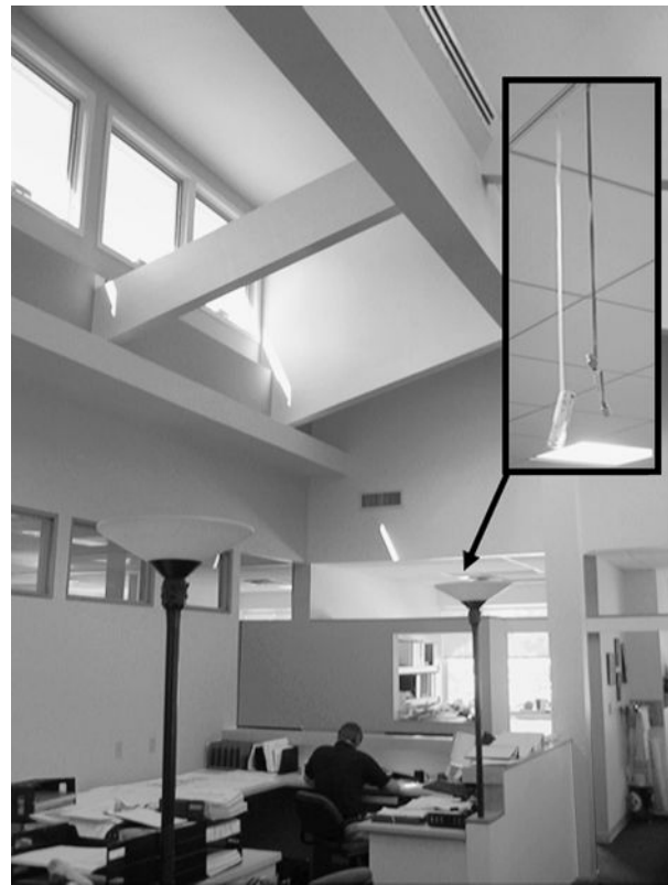
Figure 8-18 Air sampling using a test kit can identify potential indoor air quality issues. The test kit shown here draws an air sample from an area of about 1,000 square feet, which is then sent to a lab for analysis. The IAQ parameters tested, in this case, yielded results for total volatile organic compounds, formaldehyde, and mold. Image courtesy of Todd Reed.
