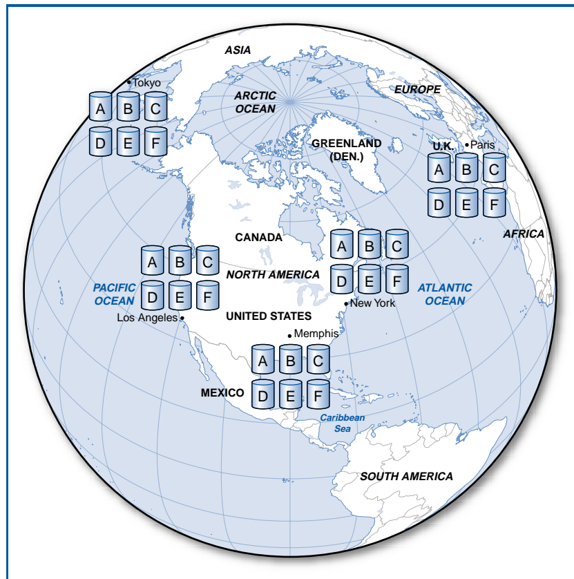
FIGURE 12.7 Distributed database with maximum data replication
