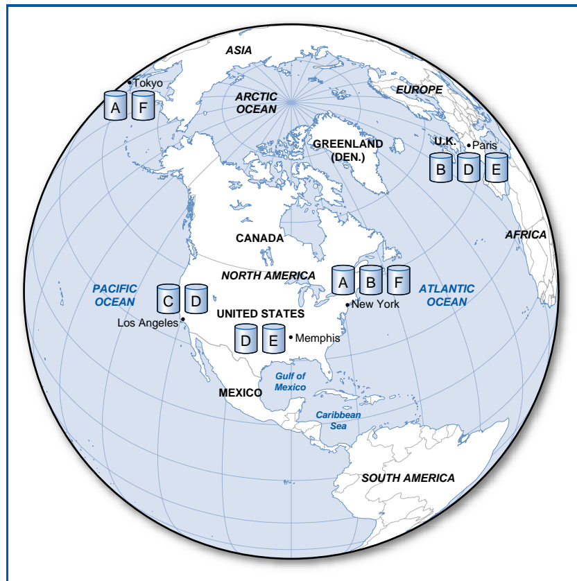
FIGURE 12.9 Distributed database with targeted data replication
