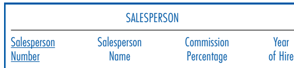
FIGURE 7.2 Conversion of an E-R diagram entity box to a relational table
