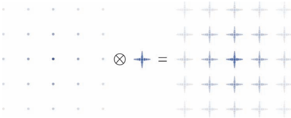
Figure 7.28 The Bragg peaks of the diffraction pattern of a nanocrystalline sample reflect the ‘shape function’ of the object.
