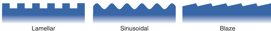
Figure 4.11 Three common grating profiles used to disperse ultraviolet light and soft x-rays.
