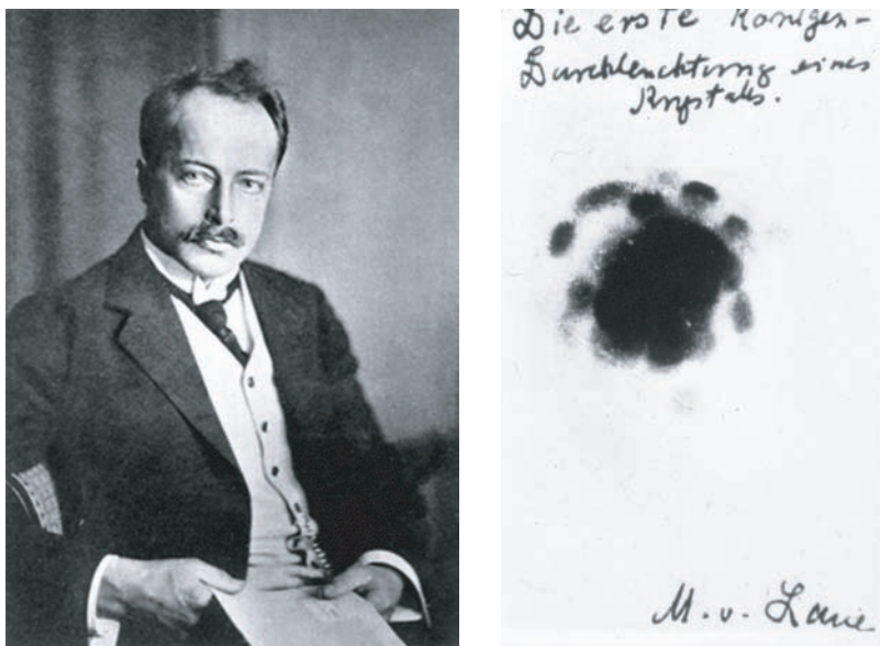
Figure 1.7 Max von Laue, and the first x-ray diffraction pattern of copper sulfate.
