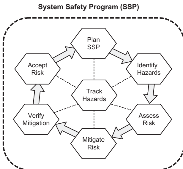
Figure 2.86 Core process, closed-loop view.
