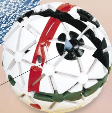
The camera is protected from collisions with other equipment by the cushioned surface.
