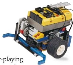
The robots are powered by batteries housed near the control panel.
