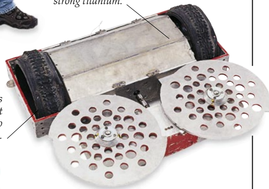
The body is made of light, strong titanium.
