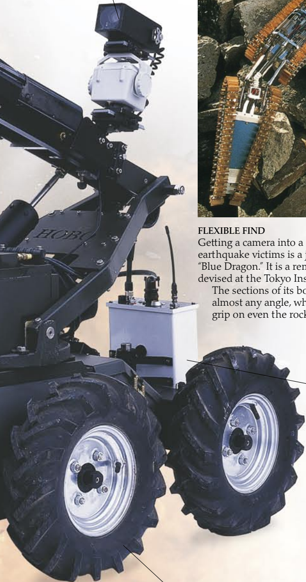
Each wheel is driven by a separate motor.
