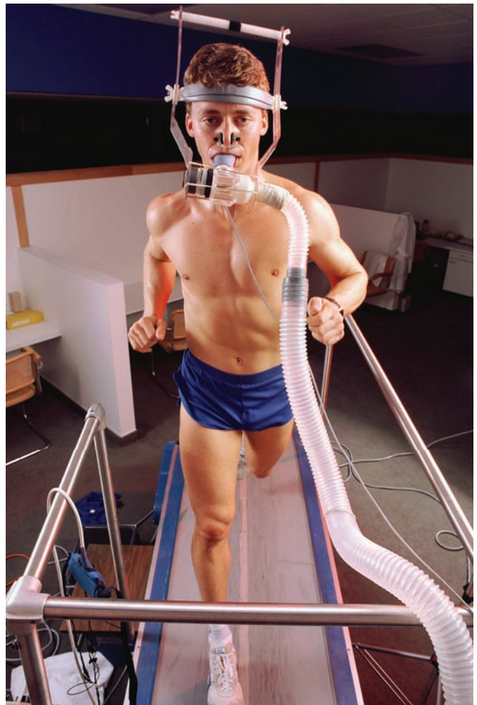
Figure 13-1. Treadmill protocols increase the workload by either increasing velocity or the percent grade. The increment in workload and how quickly workload is elevated depends on the purpose of the test.
