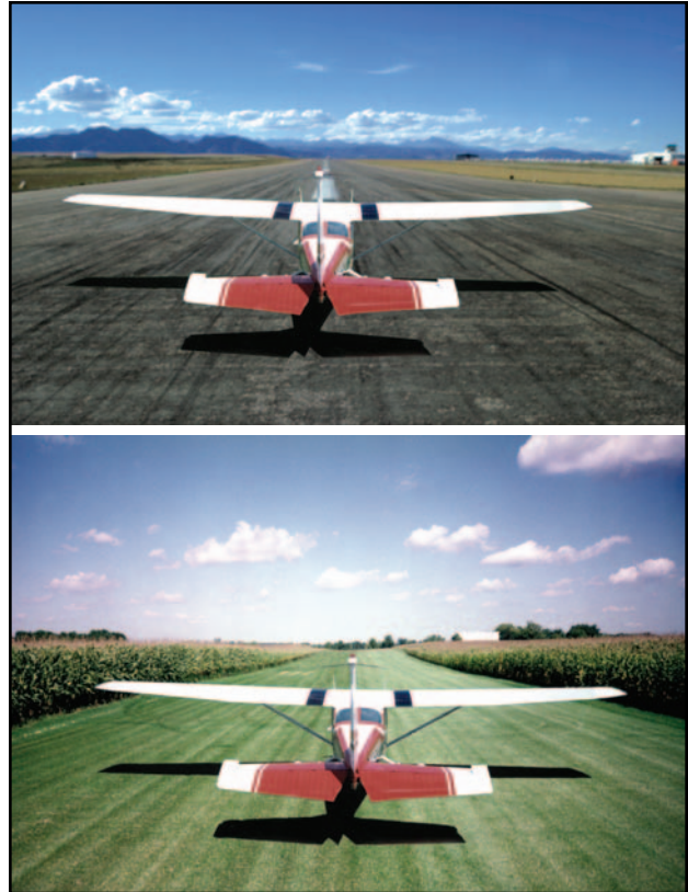
Figure 9-17. Airplane performance depends greatly on the runway surface.
