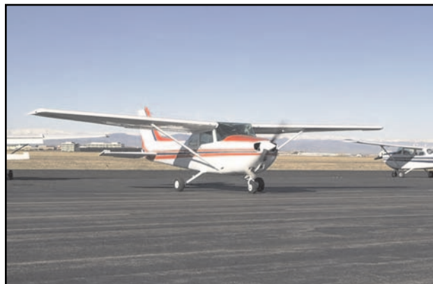
Figure 5-26. The landing gear supports the airplane during the takeoff run, landing, taxiing, and when parked.
