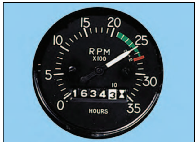
Figure 5-5. Engine r.p.m. is indicated on the tachometer.
