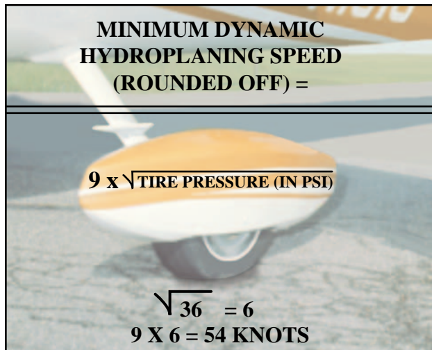
Figure 9-19. Dynamic hydroplane formula and example for a tire pressure of 36 pounds.
