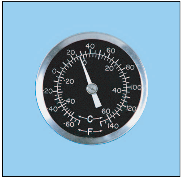
Figure 6-24. Outside air temperature gauge.
