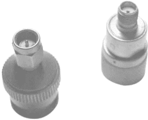
Figure 6-16. SMA: Sub-Miniature connector, variation A
