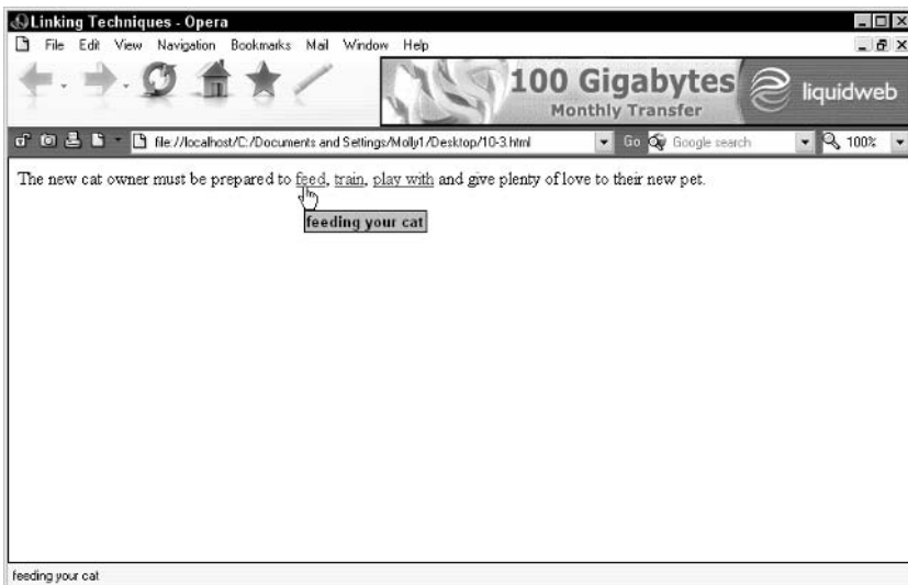
Figure 10-3: Additional title attribute information within a tool tip. Note how the Opera browser also displays the title attribute information in the browser status bar upon mouseover.
