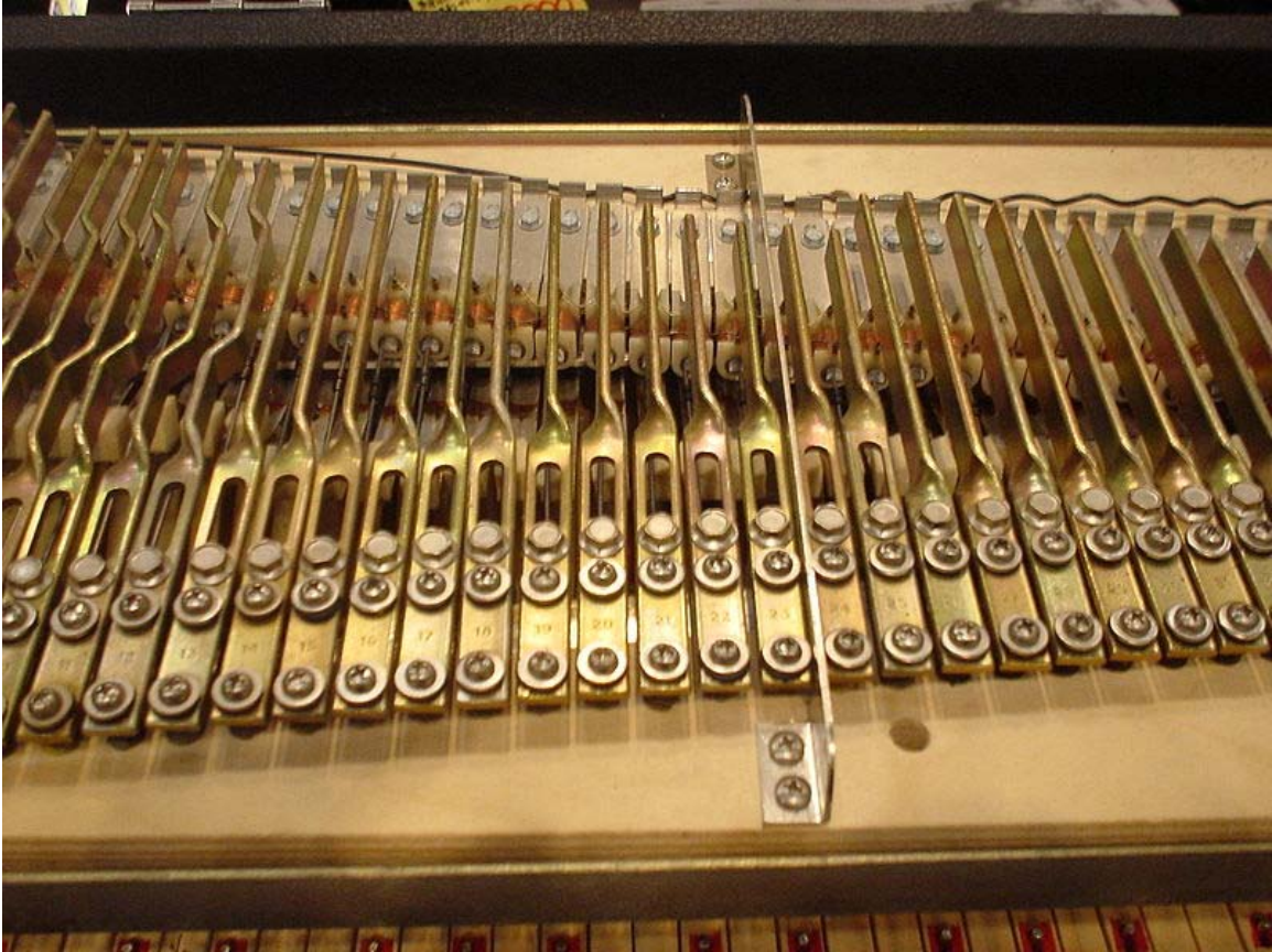
Tuning forks of Fender Rhodes Mark I
