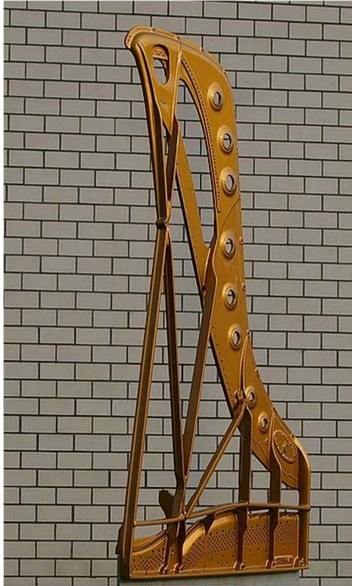
Cast iron plate of a Steinway grand piano
