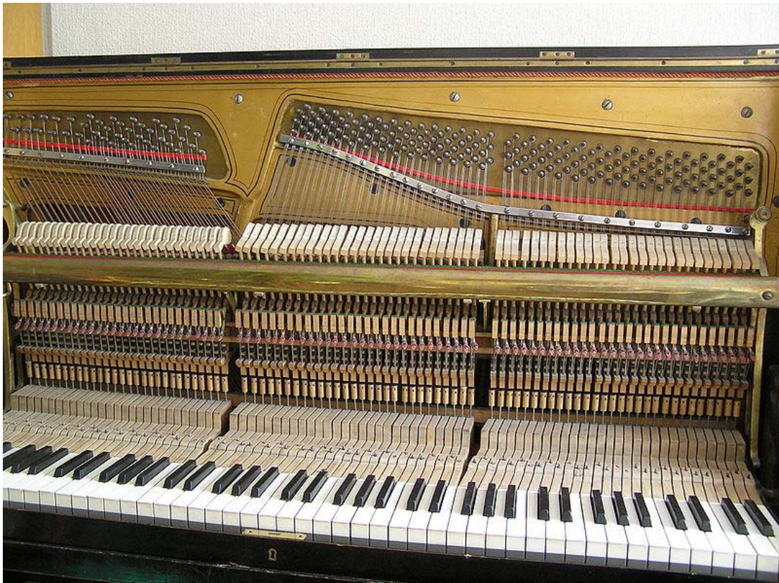
The mechanism in upright pianos is perpendicular to the keys
