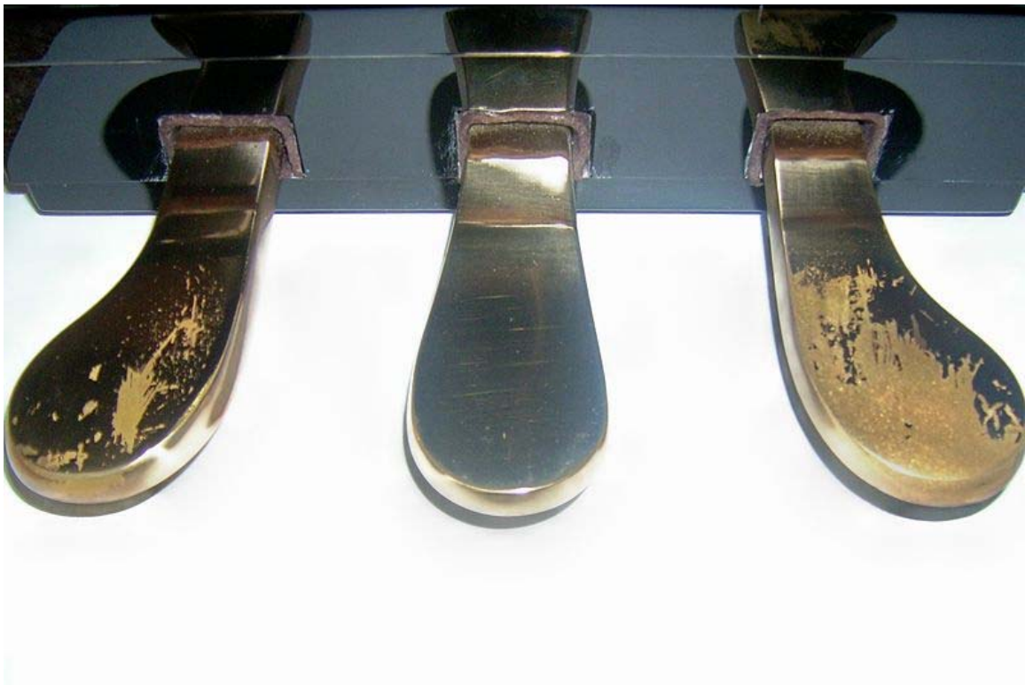
Piano pedals from left to right: una corda, sostenuto, and sustain pedal
